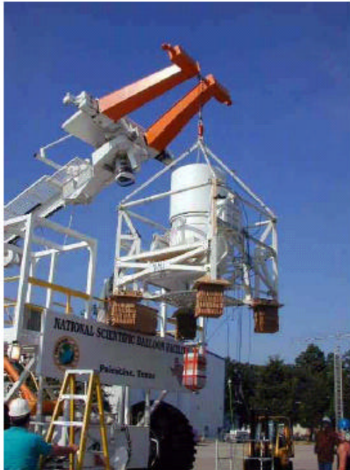
Figure 1. The GLAST Balloon Flight Engineering Model (BFEM) during testing at National Scientific Balloon Facility, Palestine, Texas.
