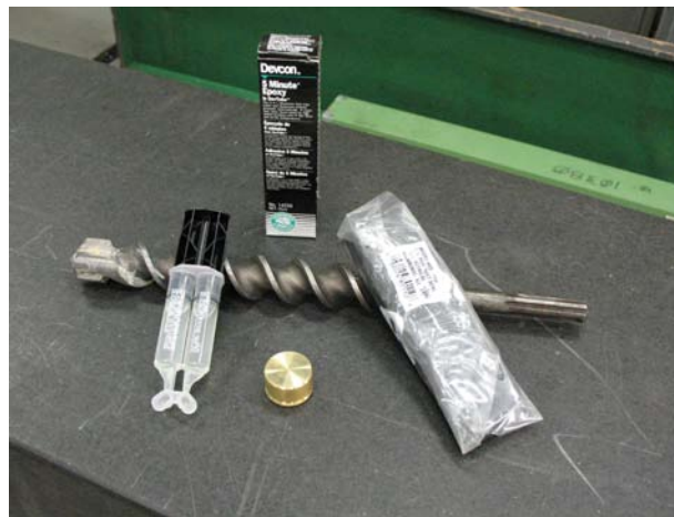
A Brass Plug with Most of the Equipment Used for Installation
