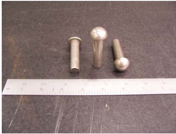
Rivets Before Installation
