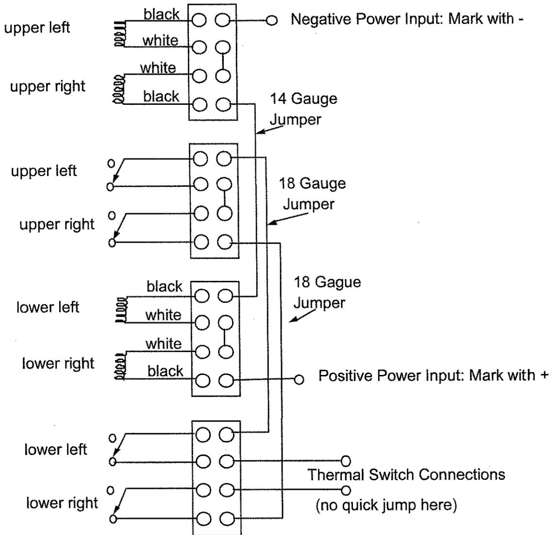
left and right refer to observer looking downstream, in the beam direction
