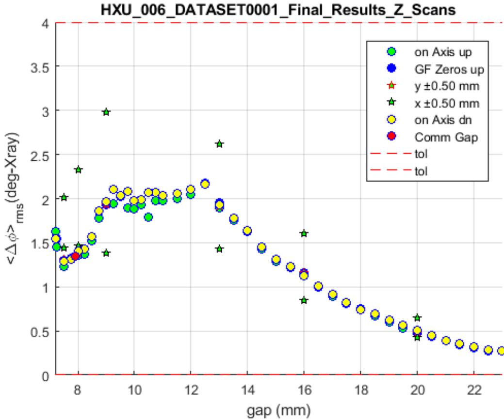
The figure shows the phase shake,  $\langle \Delta\phi \rangle_{rms}$ , (see above) as a function of operational gap. The vertical axis extends over the entire tolerance range. The values show a slight hysteresis (show explanation above) but are well within tolerance.
