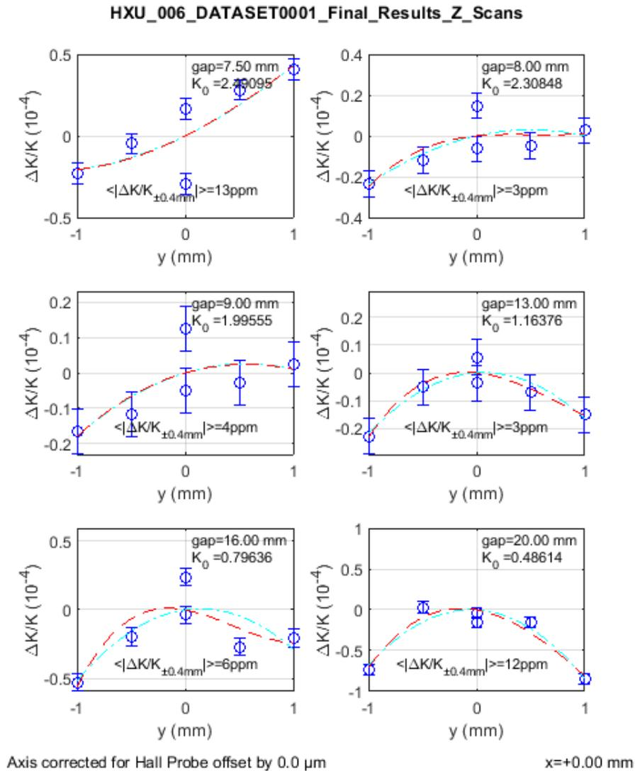
The figure shows the deviation of the relative undulator strength,  $K$ , value from the on-axis value,  $K_0$ , as function of  $y$  at a number of operational gaps. The deviations follow closely the expected functional form  $(\cosh(k_u y) - 1)$ . [Documentary Information]
