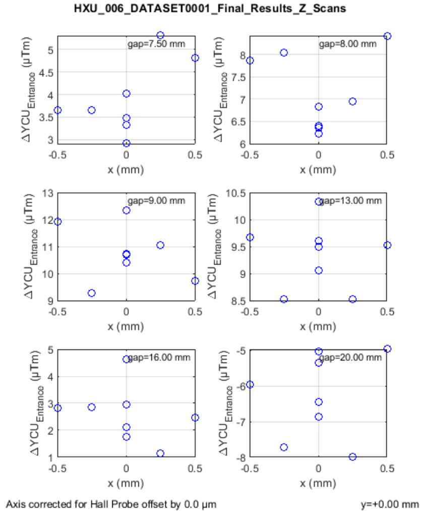
The figure shows the required strength of the upstream horizontal corrector to remove the second horizontal undulator field integral at the downstream BPM for a number of operational undulator gaps. The analysis was done at a number of off-axis locations in the x-z plane. All values are small and well below the maximum correction capabilities of greater than 550  $\mu Tm$  of the actual correctors.
