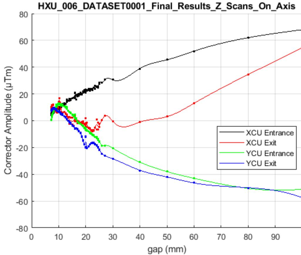
The figure shows as a function of undulator gap the required strengths of the upstream and downstream horizontal and vertical correctors to remove the effect of undulator field integrals at the downstream BPM over the entire available gap range. All values are small and well below the maximum correction capabilities of greater than 550  $\mu\text{Tm}$  of the actual correctors.
