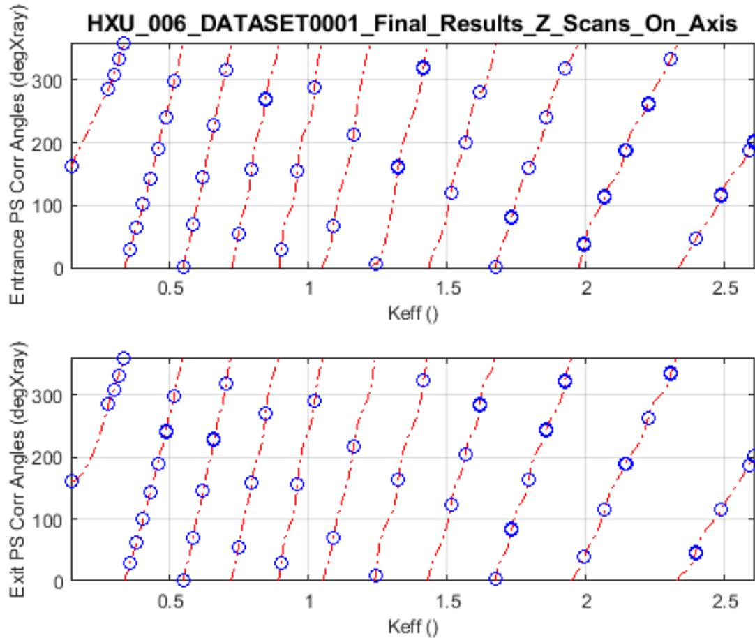
The top and bottom figures as a function of undulator parameter  $K_{eff}$  the required correction angles to be added to the upstream and downstream phase shifters, respectively. The red lines indicate the minimum required phase shifter phase angle increases, which are in the 0 to 360 degXray phase shift range. The blue circles indicate MMF measurements.
