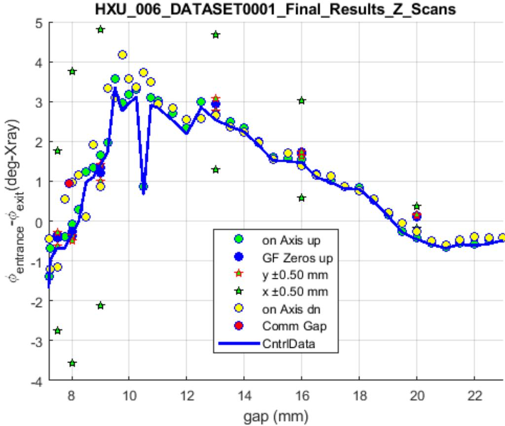
The figure shows a (negligible) imbalance of the entrance (cell boundary start to undulator core) to the exit (undulator core to cell boundary end) phase slippage for the undulator. In addition to the signals described above, the blue curve is a spline fit to the difference of the data in files
