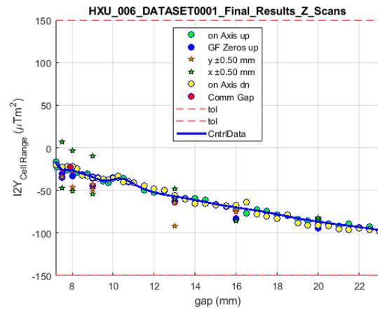
The figures show the field integrals ( $I1X$ ,  $I2X$ ,  $I1Y$ ,  $I2Y$ ) as function of the operational gap. The proximity of the green and yellow circles shows that the field integrals are not sensitive to the hysteresis in  $K$  as seen on a previous page. The blue curves are spline fits to the data in files
