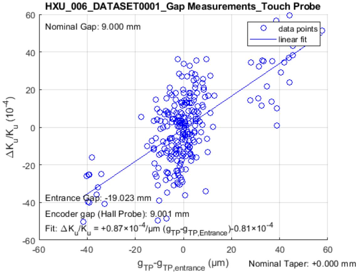
The figure shows the correlation between the  $\Delta K_u / K_u$  for each pole from Hall probe measurements for the tuning gap and the deviation of the pole gap measured by the touch probe relative to its average (for the 246 core poles). The average gap measured with the touch probe and the one measured with the gap encoder are shown in the lower left corner of the figure. Also shown is the fit function.
