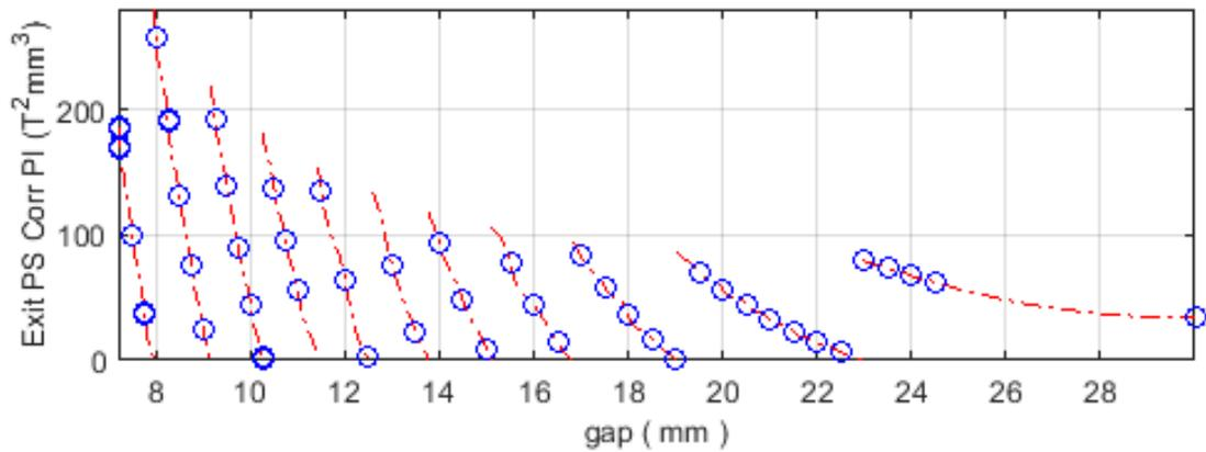
The top and bottom figures show as a function of undulator gap the required correction phase integral (PI) values to be added to the upstream and downstream phase shifters, respectively. The red lines indicate the minimum required phase shifter phase angle increases, which are in the 0 to 360 degXray phase shift range. The blue circles indicate MMF measurements.
