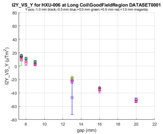
The figure shows the field integrals obtained from long coil measurements off axis in the horizontal plane using colors to indicate offset distance (black: -1.0 mm, blue: -0.5 mm, green: on-axis; red: +0.5 mm, magenta: +1.0 mm). The vertical axes extend over the tolerance range. All integrals are in tolerance.
