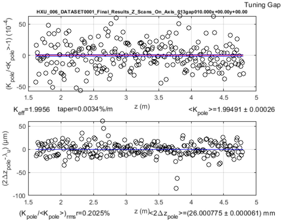
The figures show the per-pole undulator strength  $K_{pole}$  (upper) and the deviation of the pole width from the expected value of  $\lambda_u/2$  (lower) for the 246 core undulator poles for the tuning gap. The horizontal lines indicate the mean (center red line) and the rms deviations from the mean (two black lines above and below the average). The corresponding mean and rms values are also printed on the right hand side underneath each figure. [Documentary Information]
