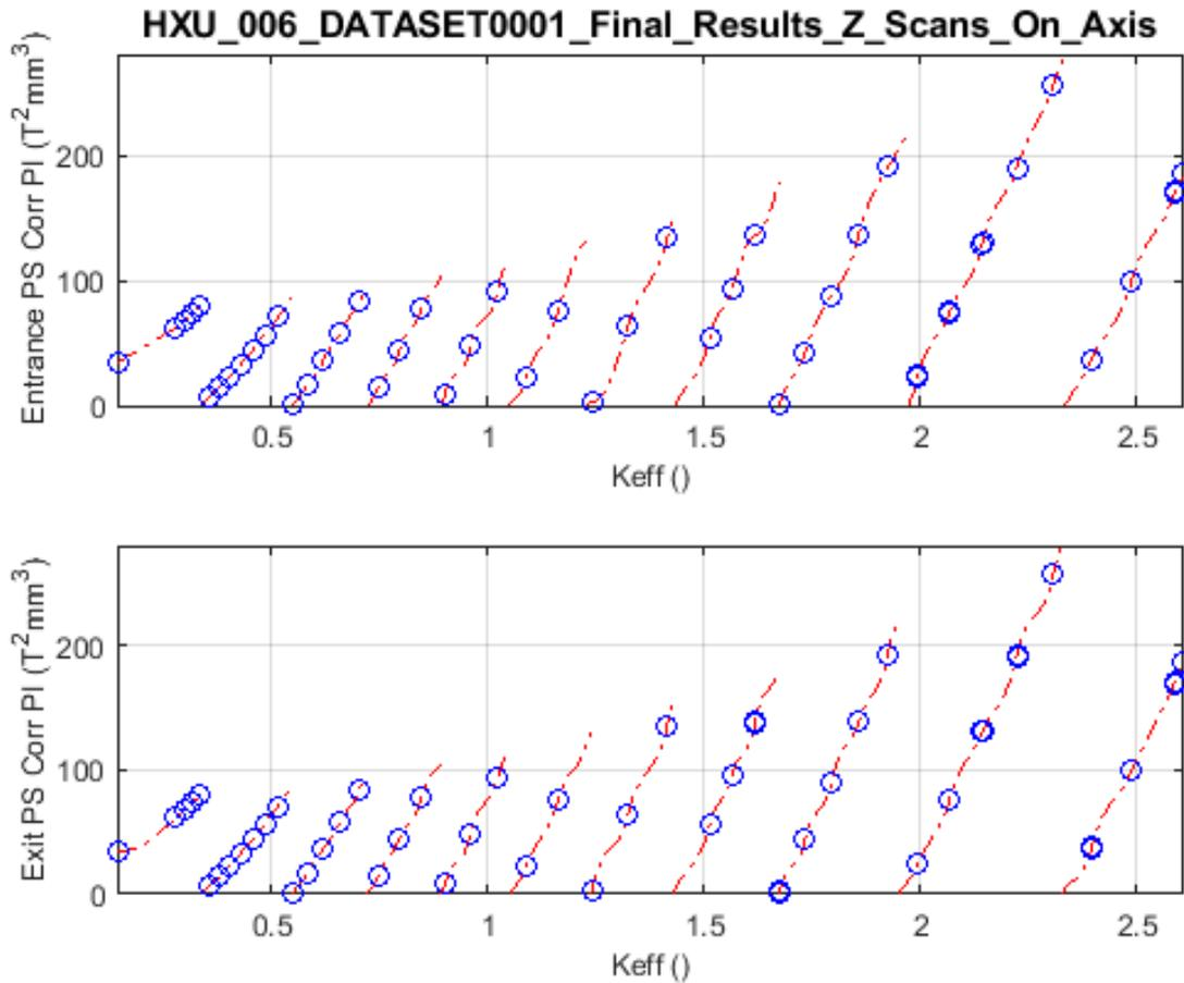
The top and bottom figures show as a function of undulator parameter  $K_{eff}$  the required correction phase integral (PI) values to be added to the upstream and downstream phase shifters, respectively. The red lines indicate the minimum required phase shifter phase angle increases, which are in the 0 to 360 degXray phase shift range. The blue circles indicate MMF measurements.
