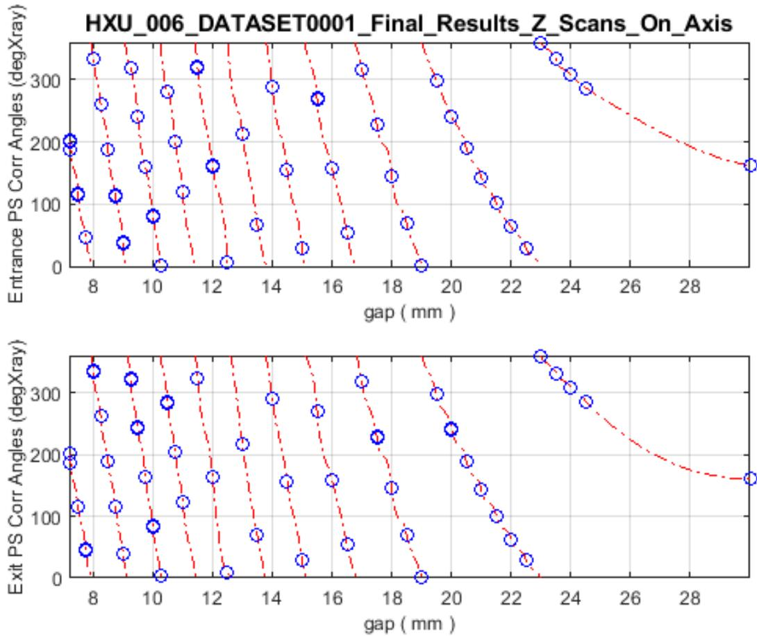
The top and bottom figures show as a function of undulator gap the required correction angles to be added to the upstream and downstream phase shifters, respectively. The red lines indicate the minimum required phase shifter phase angle increases, which are in the 0 to 360 degXray phase shift range. The blue circles indicate MMF measurements.
