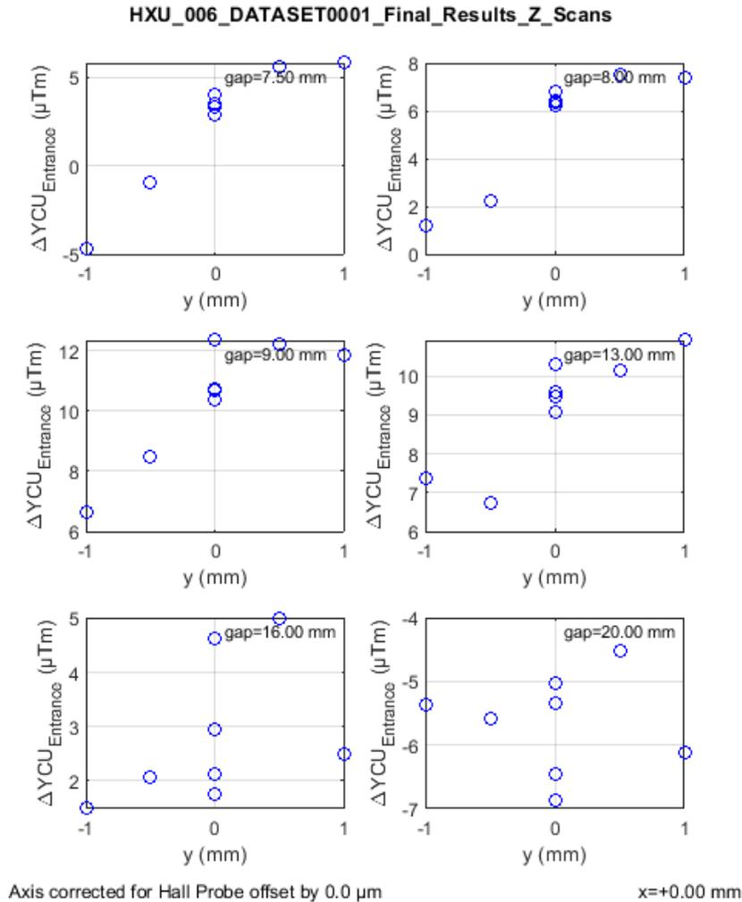
The figure shows the required strength of the upstream vertical corrector to remove the second horizontal undulator field integral at the downstream BPM for a number of operational undulator gaps. The analysis was done at a number of off-axis locations in the  $y$ - $z$  plane. All values are small and well below the maximum correction capabilities of greater than 550  $\mu Tm$  of the actual correctors.
