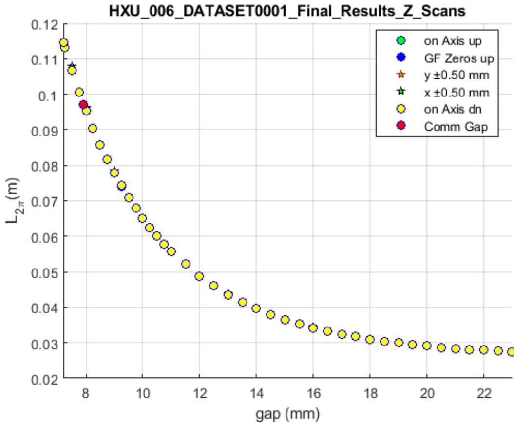
The figure shows the free space distance over which a  $2\pi$  slippage occurs between the radiation field and the electron bunch (see explanation above) as a function of undulator gap over the operational gap range. Note: the free space travel distance required to accumulate  $2\pi$  slippage gets shorter towards larger gap values, which correspond to shorter undulator wavelengths. [Documentary Information]
