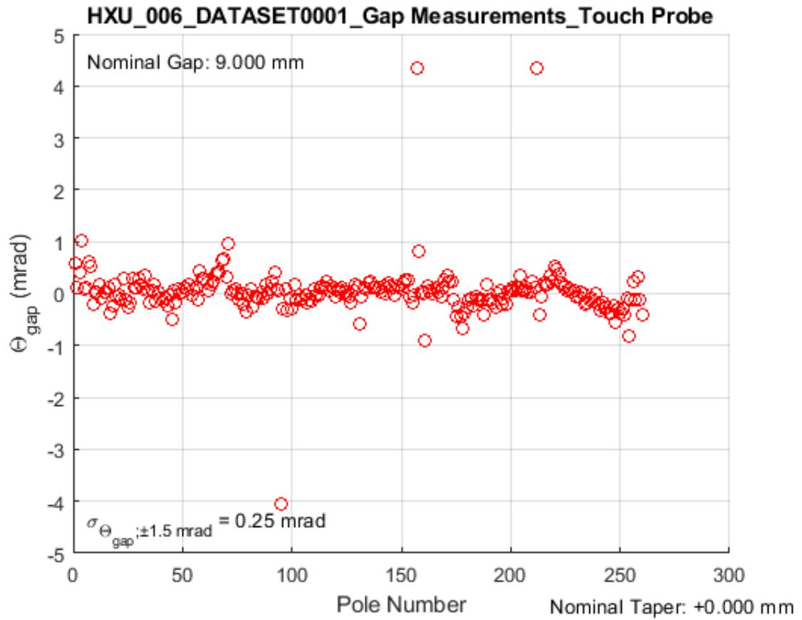
The figure shows the cant angles between the top and bottom part of each pole at the Tuning Gap for all 260 poles, measured by the touch probe. The rms width of each distribution within a  $\pm 1.5$  mrad band is shown in the lower left corner of the figure.
