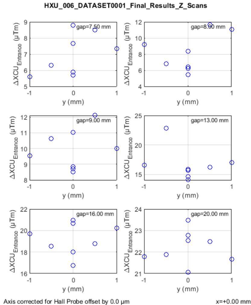
The figure shows the required strength of the upstream horizontal corrector to remove the second vertical undulator field integrals at the downstream BPM for a number of operational undulator gaps. The analysis was done at a number of off-axis locations in the  $y$ - $z$  plane. All values are small and well below the maximum correction capabilities of greater than  $550 \mu Tm$  of the actual correctors.
