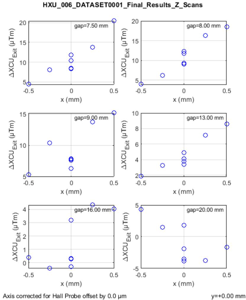
The figure shows the required strength of the downstream horizontal corrector to remove the first vertical undulator field integral and upstream corrector field integral at the downstream BPM for a number of operational undulator gaps. The analysis was done at a number of off-axis locations in the x-z plane. All values are small and well below the maximum correction capabilities of greater than 550  $\mu Tm$  of the actual correctors.
