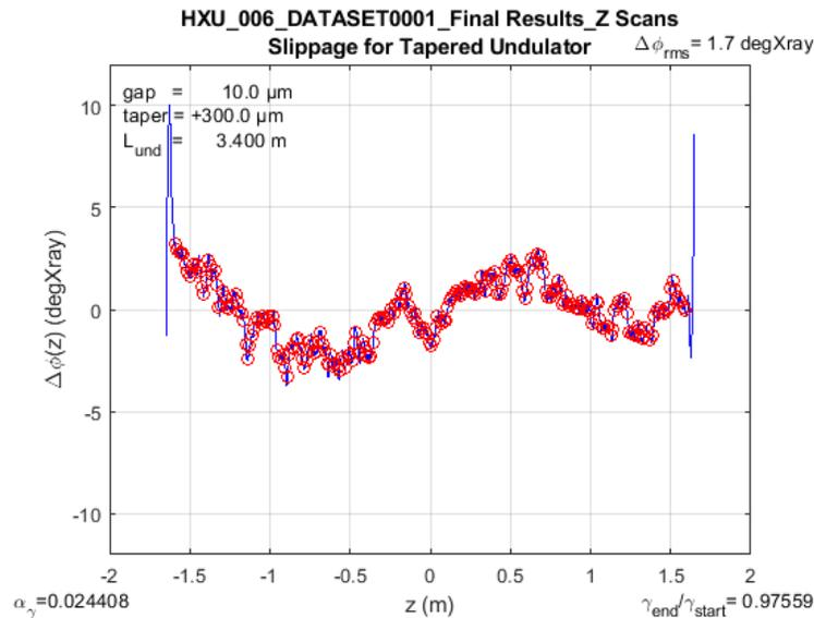
The upper figure shows a simplified linear energy loss function (Lorentz factor  $\gamma/\gamma_{Start}$ ) optimized for the 0.3 mm gap taper at an 10 mm nominal gap. The lower figure shows the phase error along the undulator segment for the same parameters.
