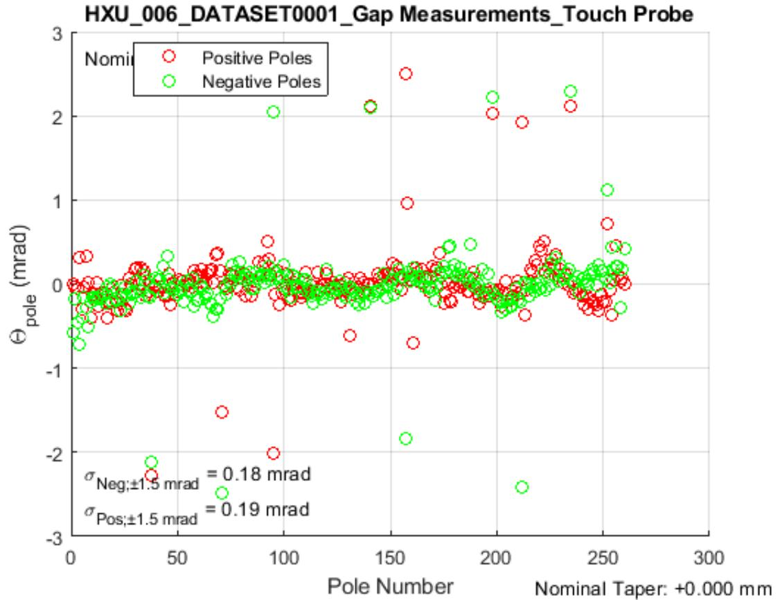
The figure shows the cant angles of each pole (top red, bottom green) relative to the horizontal plane defined by the Kugler bench at the Tuning Gap for all 260 poles, measured by the touch probe. The rms width of each distribution within a  $\pm 1.5$  mrad band is shown in the lower left corner of the figure.
