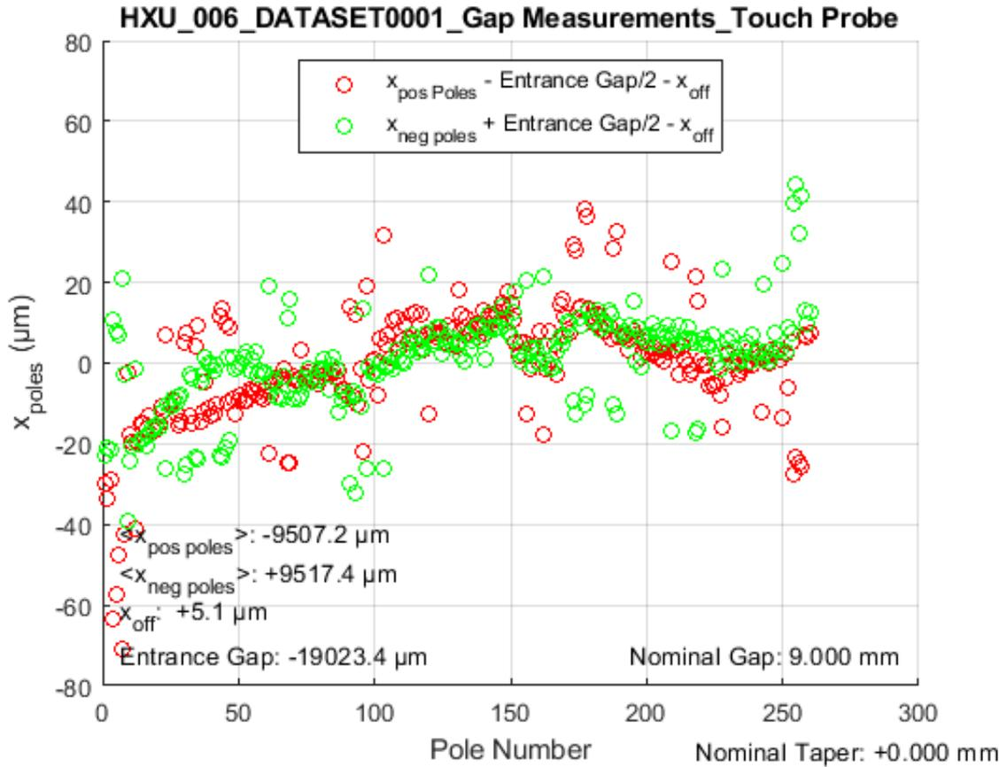
The figure shows the relative vertical positions of the center of each pole (top red, bottom green) relative to the horizontal plane define by the Kugler bench at the Tuning Gap for all 260 poles, measured by the touch probe.
