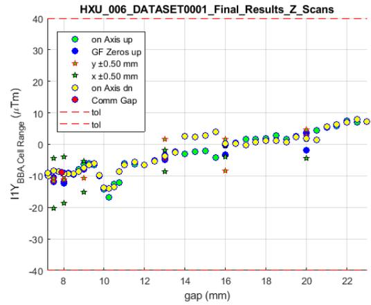
The figure shows the first integrals after a BBA equivalent correction was applied. The values stay within tolerance over the operational range.
