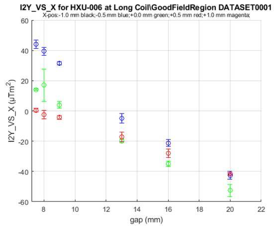
The figure shows the integrals obtained from long coil measurements off axis in the vertical plane using colors to indicate offset distance (black: -1.0 mm, blue: -0.5 mm, green: on-axis; red: +0.5 mm, magenta: +1.0 mm). The vertical axes extend of the tolerance range. All integrals are in tolerance.
