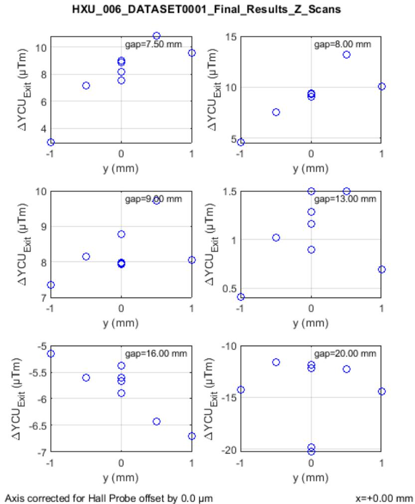
The figure shows the required strength of the downstream vertical corrector to remove the first horizontal undulator field integral and the upstream corrector field integral at the downstream BPM for a number of operational undulator gaps. The analysis was done at a number of off-axis locations in the  $y$ - $z$  plane. All values are small and well below the maximum correction capabilities of greater than  $550 \mu\text{Tm}$  of the actual correctors.
