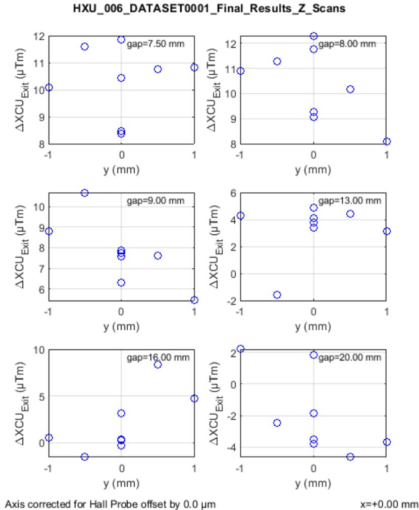
The figure shows the required strength of the upstream horizontal corrector to remove the first vertical undulator and upstream corrector field integrals at the downstream BPM for a number of operational undulator gaps. The analysis was done at a number of off-axis locations in the  $y$ - $z$  plane. All values are small and well below the maximum correction amplitude of greater than 550  $\mu Tm$  capabilities of the actual correctors.
