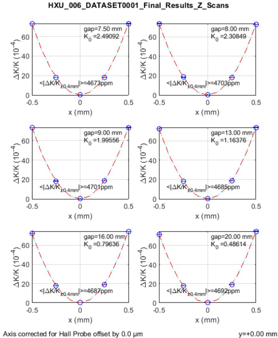
The figure shows the deviation of the relative undulator strength,  $K$ , from the off-axis value,  $K_0$ , as function of  $x$  at a number of operational gaps. The average deviation at  $z = 0.4$  mm is well below the tolerance of 160 ppm in all cases.
