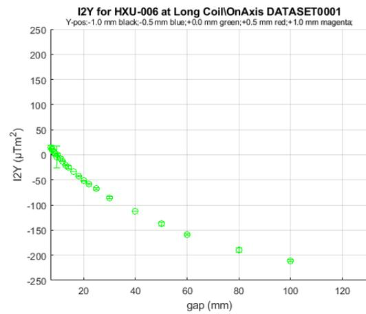
The figure shows the field integrals obtained from long coil measurements on-axis. The vertical axes extend over the tolerance range. All integrals are in tolerance.
