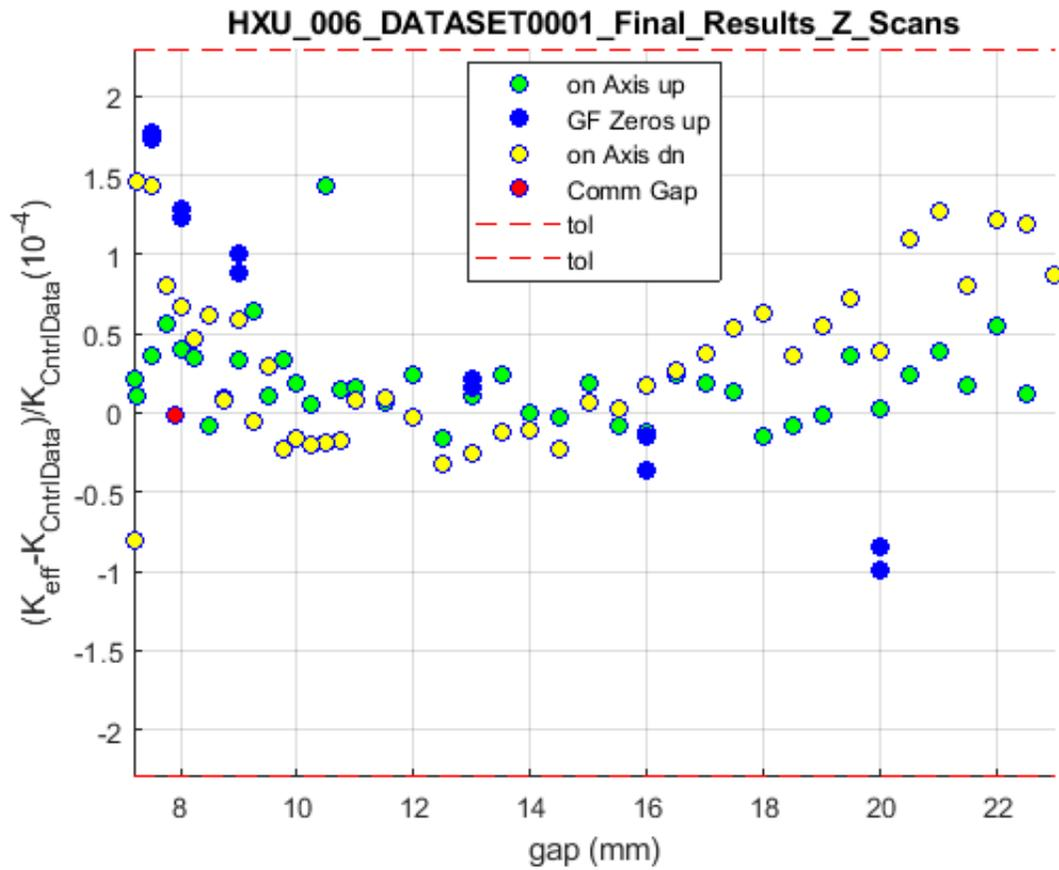
The figure shows some of the data shown in the previous figure but with a larger vertical scale that just captures the tolerance range. The off-axis measurements are not shown.
