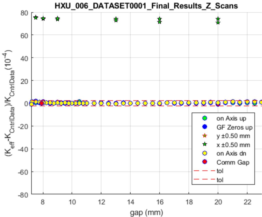
The figure shows the relative difference between the measured undulator strength  $K_{\text{eff}}$  and a cubic spline fit to the list of reference data points stored in file `hxu_006_k_vs_gap_spline.dat` in the Controls Data folder on the V: drive as a function of gap over the 7.2 mm—20 mm operational range.
