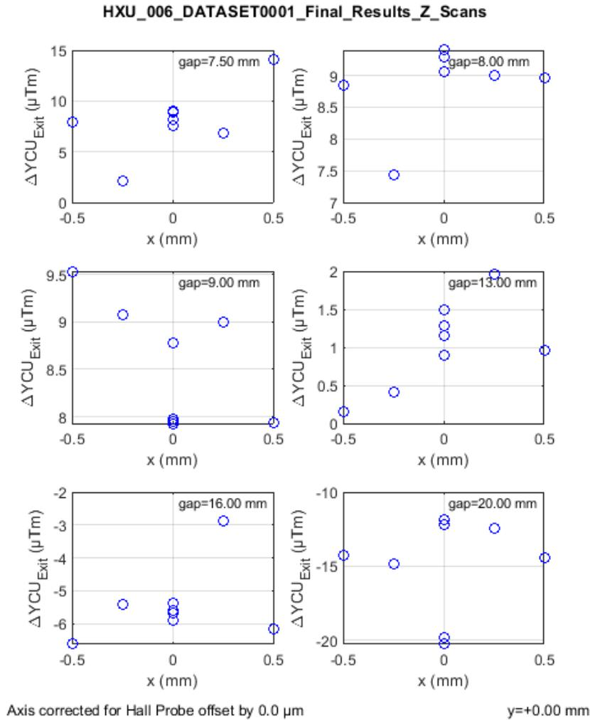
The figure shows the required strength of the downstream vertical corrector to remove the first horizontal undulator field integral and upstream corrector field integral at the downstream BPM for a number of operational undulator gaps. The analysis was done at a number of off-axis locations in the x-z plane. All values are small and well below the maximum correction capabilities of greater than 550  $\mu Tm$  of the actual correctors.
