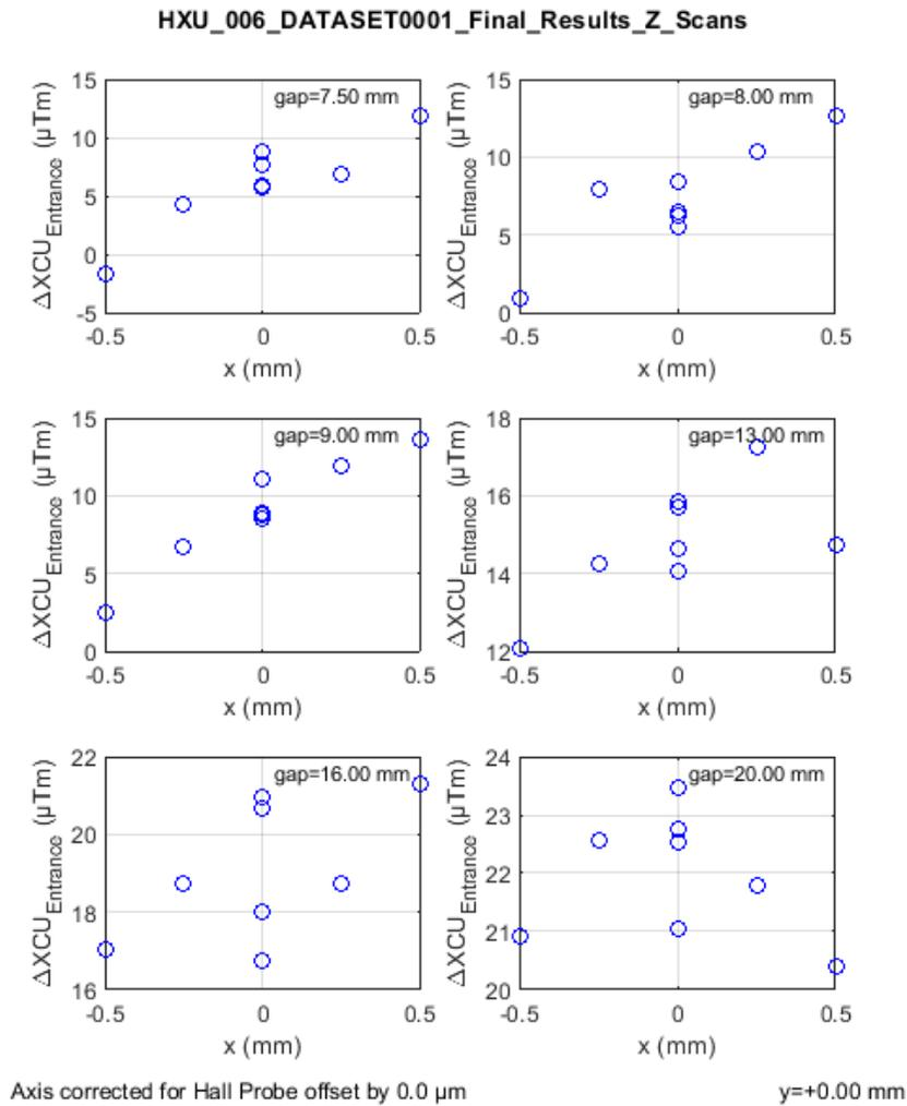
The figure shows the required strength of the upstream horizontal corrector to remove the second vertical undulator field integral at the downstream BPM for a number of operational undulator gaps. The analysis was done at a number of off-axis locations in the x-z plane. All values are small and well below the maximum correction capabilities of greater than 550  $\mu Tm$  of the actual correctors.
