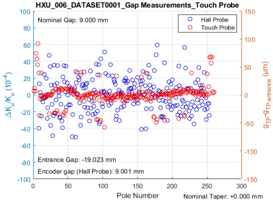
The figure shows  $\Delta K/K$  (blue, left axis) (for the 246 core poles) as well as mechanical gap heights ( $\langle g_{TP} \rangle - g_{TP}$ ) (red, right axis) (for all 260 poles) based on touch probe measurements versus pole number. The large amplitude outliers are the result of tuning.
