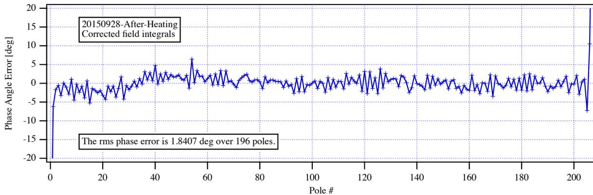
Figure 16: The measured fields, angles, trajectories and phase errors for the HXU-32 at 25 mm gap with the beam path corrected by virtual coils.
