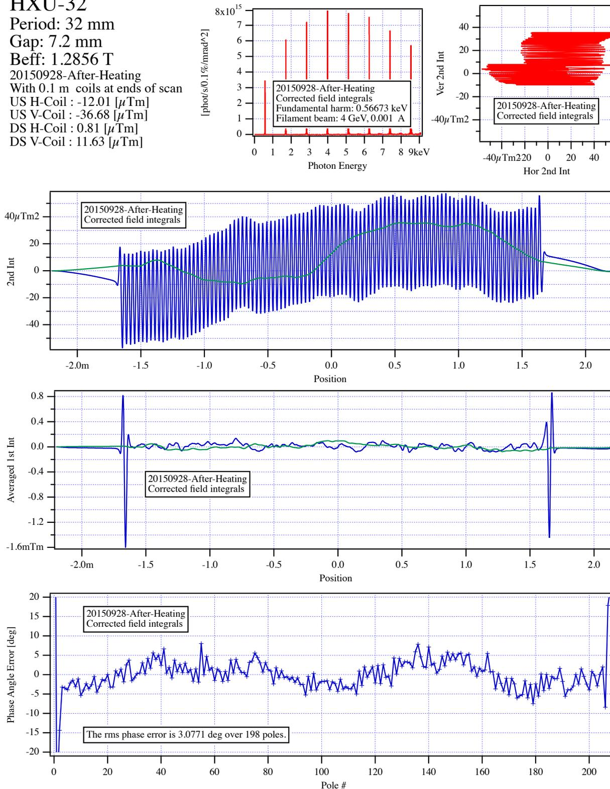
Figure 6: The measured fields, angles, trajectories and phase errors for the HXU-32 at 7.2 mm gap with the beam path corrected by virtual coils.
