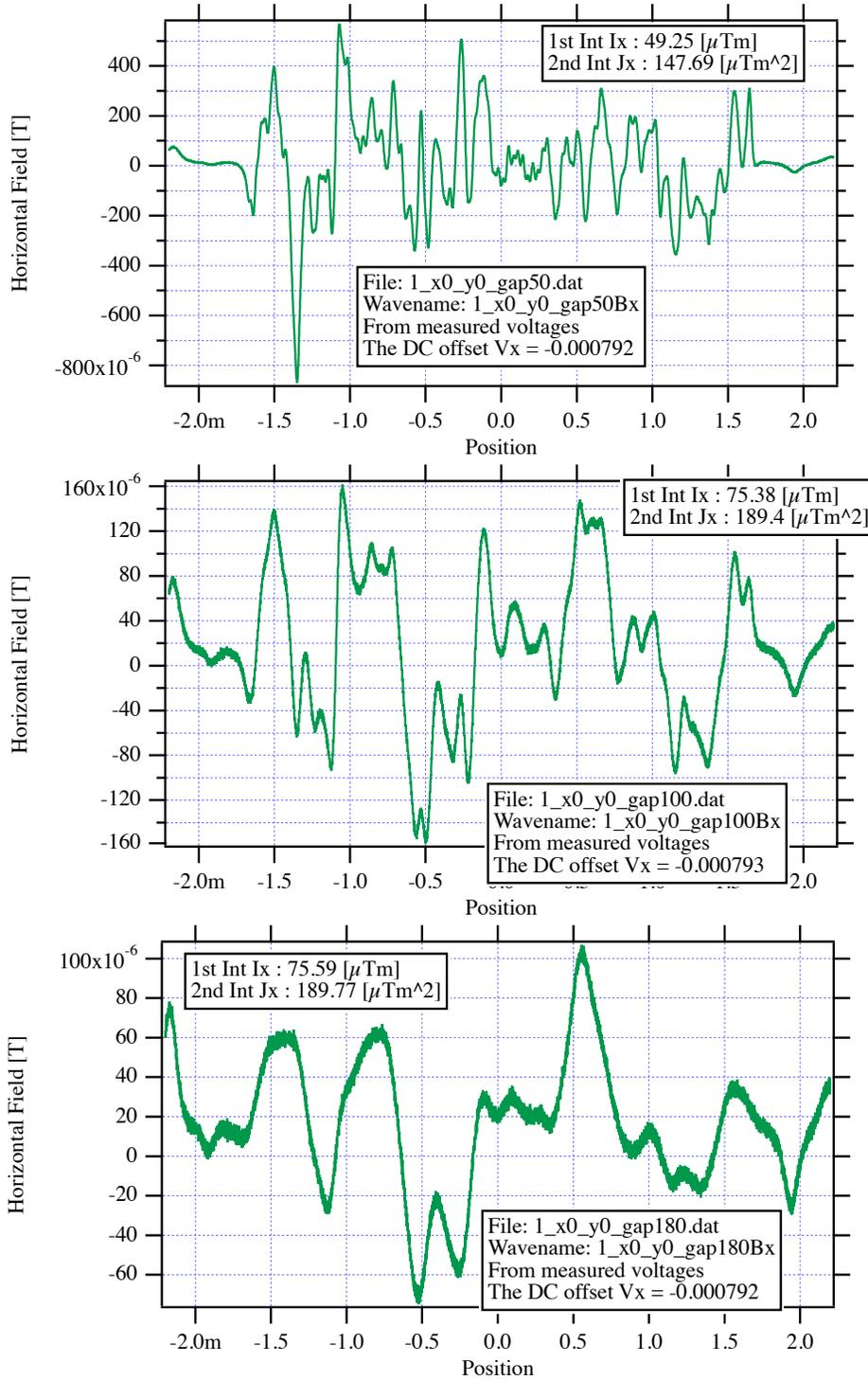
Figure 18: The measured horizontal fields for the HXU-32 at the gaps 50, 100 and 180 mm.
