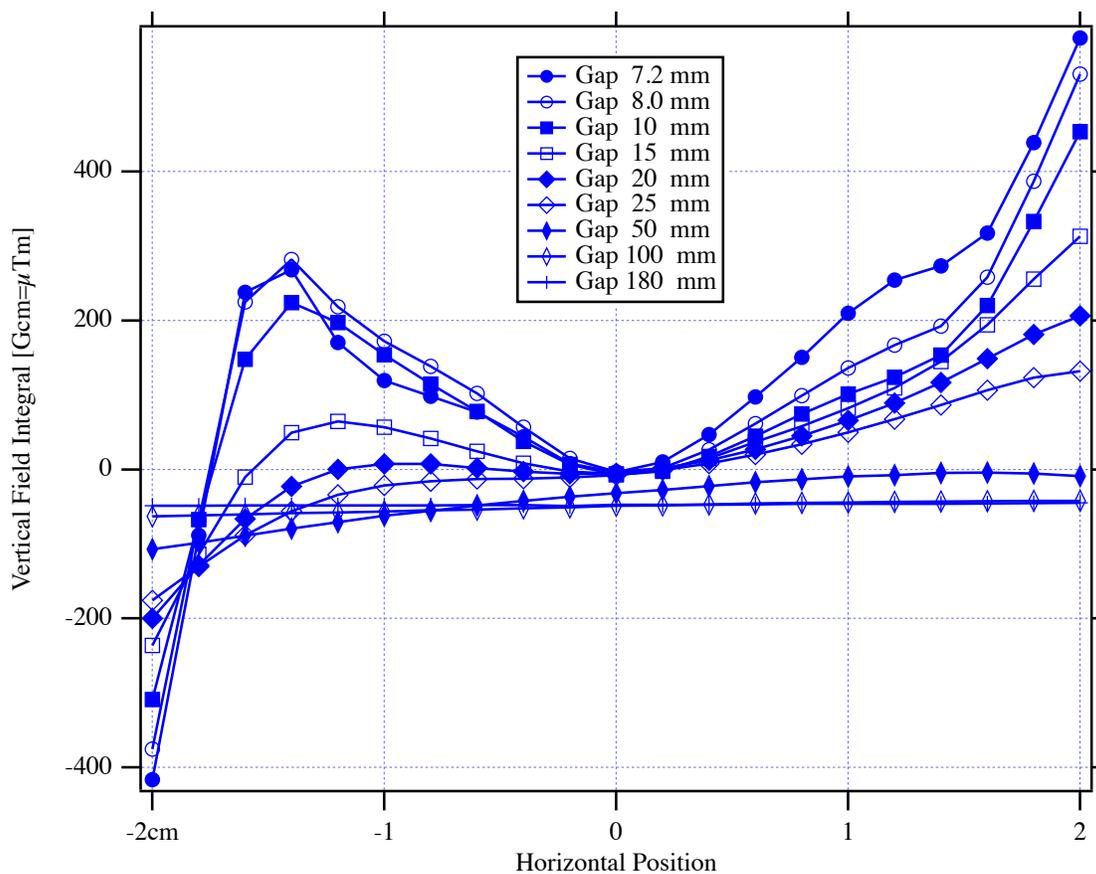
Figure 3: Vertical field integrals measured with a 3.735 m long flip coil.
