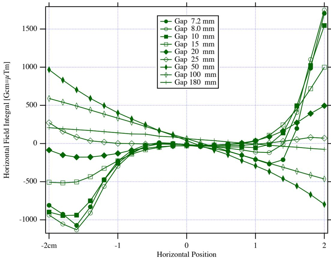
Figure 4: Horizontal field integrals measured with a 3.735 m long flip coil.
