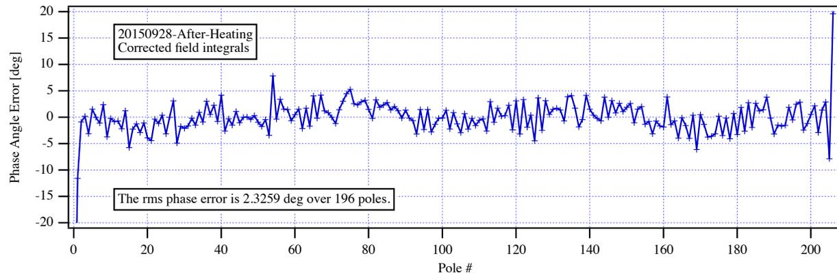
Figure 12: The measured fields, angles, trajectories and phase errors for the HXU-32 at 15 mm gap with the beam path corrected by virtual coils.
