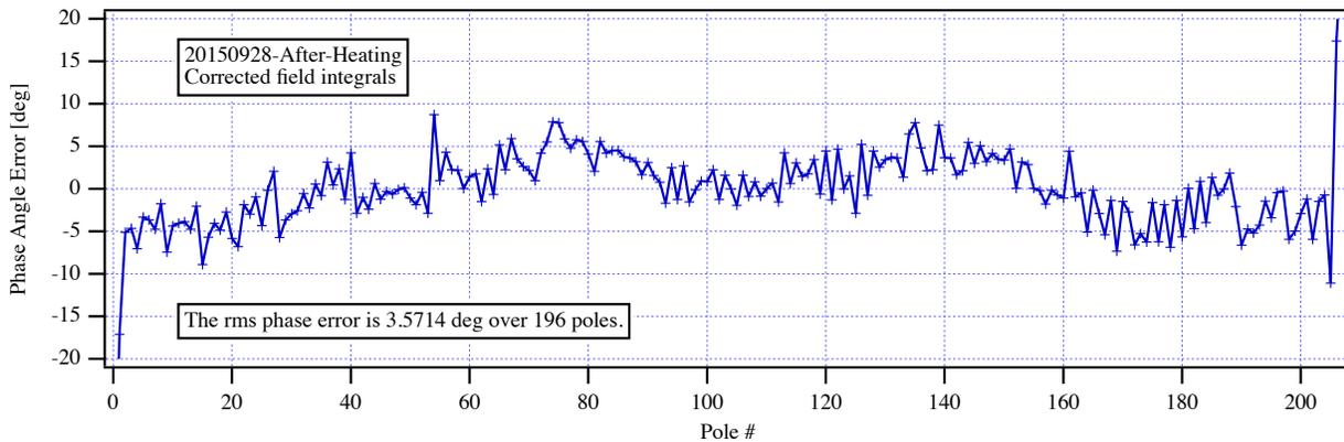
Figure 10: The measured fields, angles, trajectories and phase errors for the HXU-32 at 10 mm gap with the beam path corrected by virtual coils.
