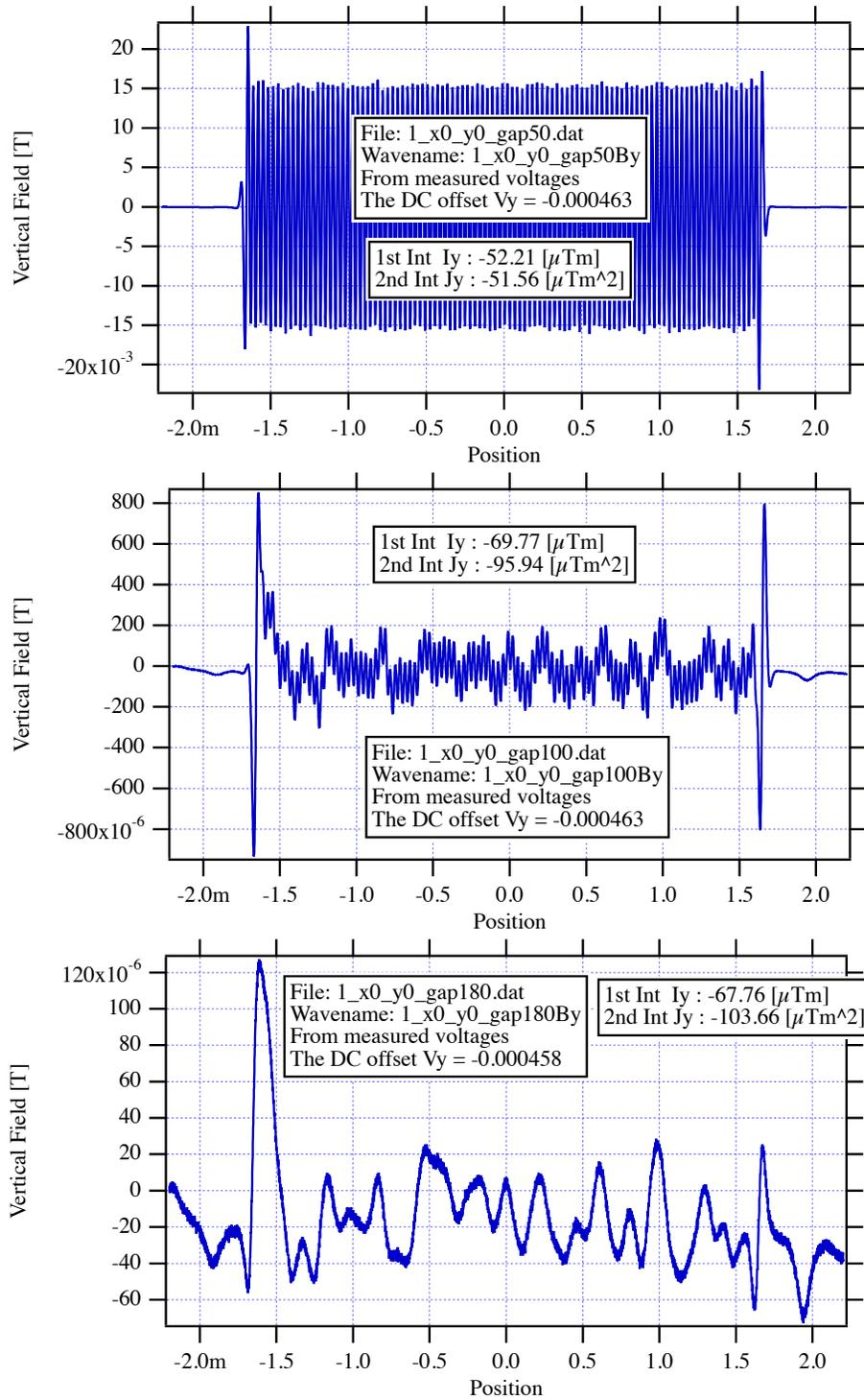
Figure 17: The measured vertical fields for the HXU-32 at the gaps 50, 100 and 180 mm.
