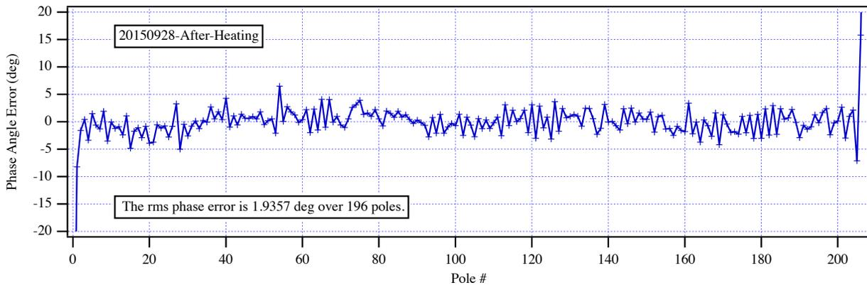
Figure 13: The measured fields, angles, trajectories and phase errors for the HXU-32 at 20 mm gap.
