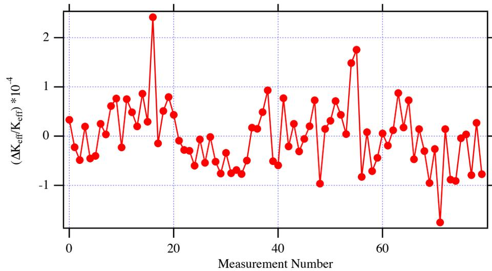
Figure 21: The measured deviation of the effective field at the repeatability measurements.
