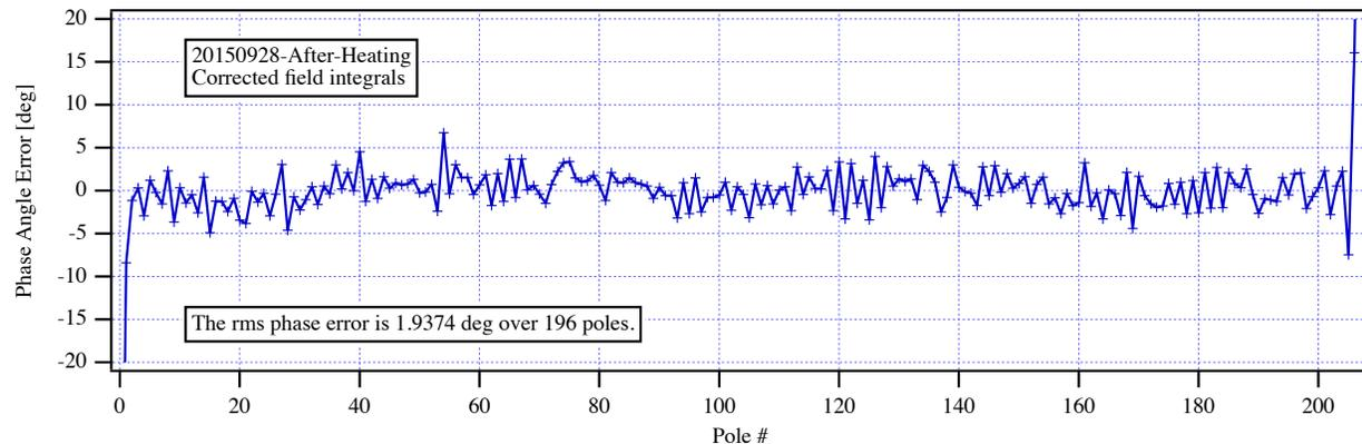
Figure 14: The measured fields, angles, trajectories and phase errors for the HXU-32 at 20 mm gap with the beam path corrected by virtual coils.
