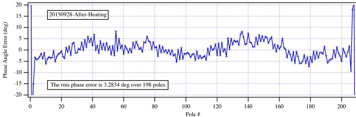
Figure 5: The measured fields, angles, trajectories and phase errors for the HXU-32 at 7.2 mm gap.
