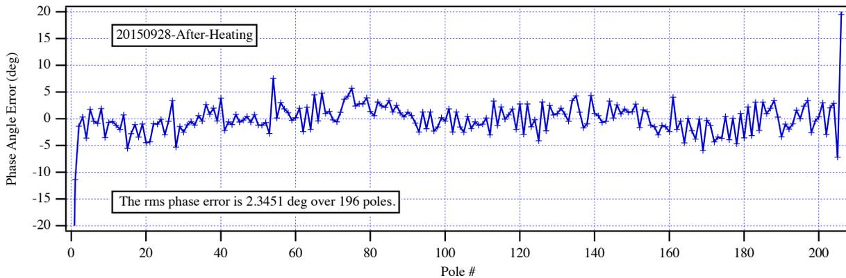
Figure 11: The measured fields, angles, trajectories and phase errors for the HXU-32 at 15 mm gap.
