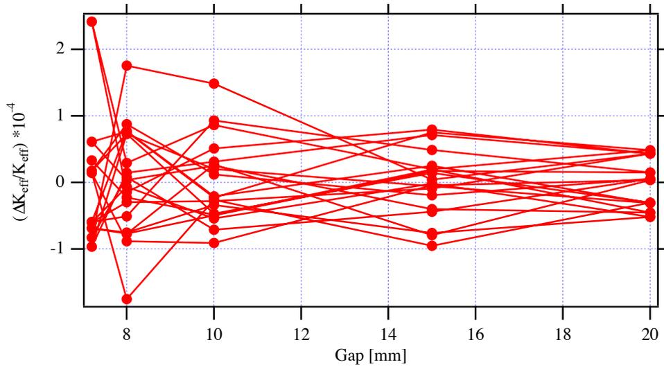
Figure 22: The measured deviation of the effective field at the repeatability measurements as a function of the gap.
