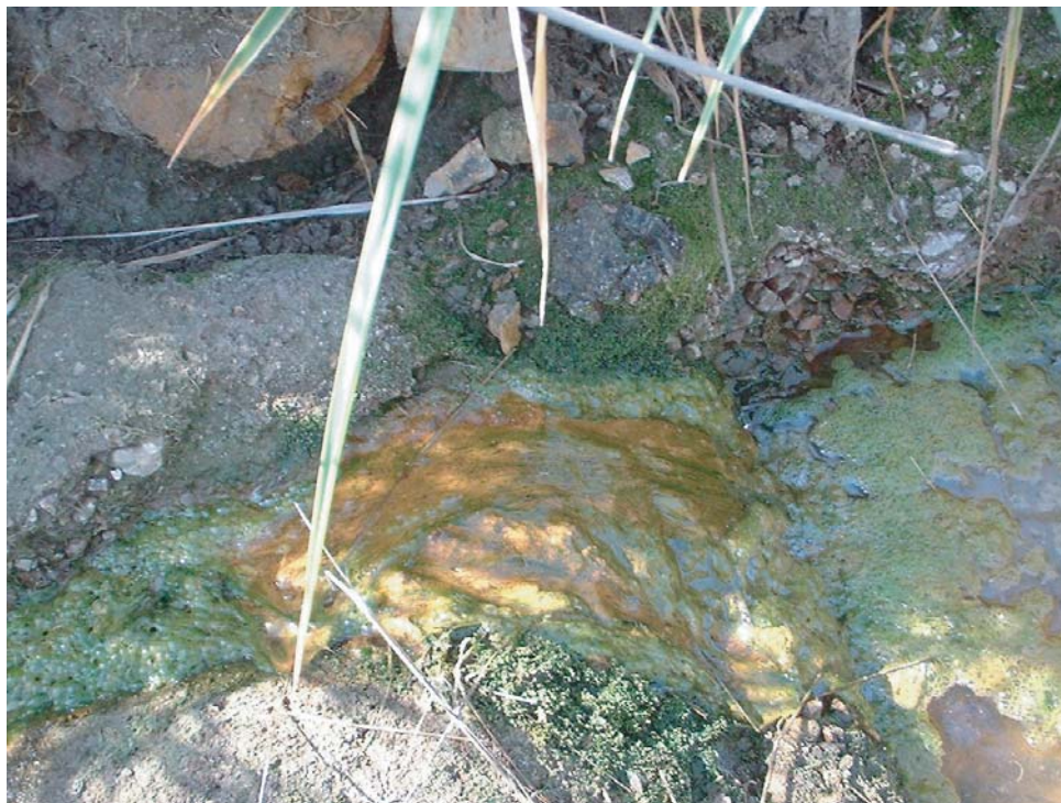
Figure 14b. Groundwater seep in Miocene-aged fractured claystone, south side of Clean Landfill
