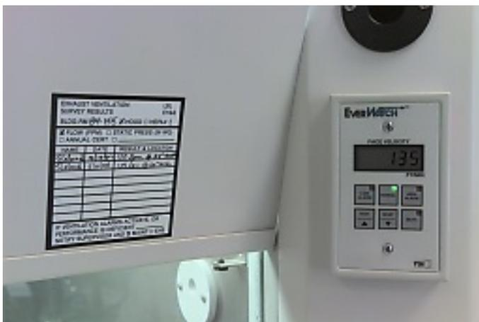
Figure 3 Quantitative Airflow Monitor and Testing Record Sticker
