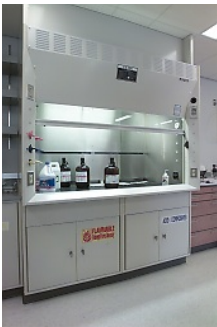
Figure 1 Laboratory Fume Hood
