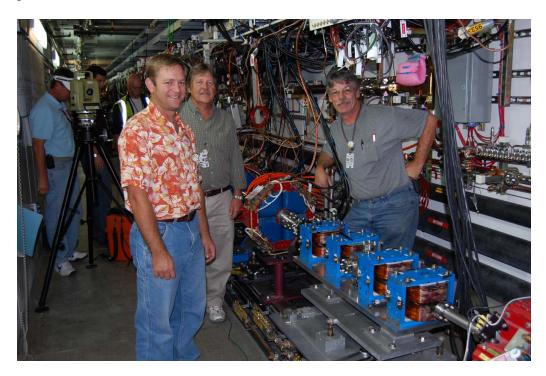
During the same time we moved all quadrupole magnets to their final locations and installed an X-band acceleration structure to raise the beam energy to 120 MeV. The MFD vacuum technicians Miguel Pinillos and Terry McCaffrey spend a whole week helping us tying all the vacuum parts back together.
