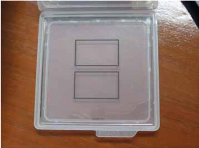
Photolithography mask for sensor coating at GOAL
