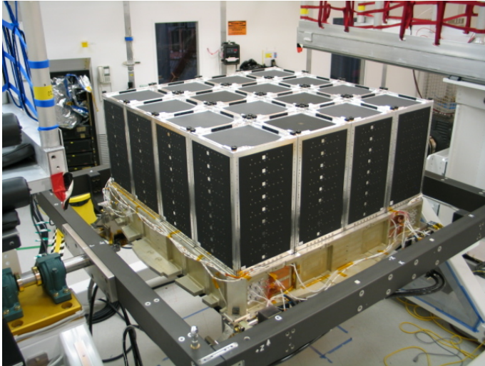
Figure 1. 16 towers installed on the LAT
