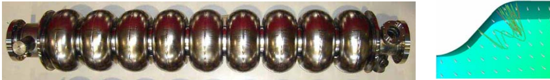
Figure 7: (Left) 9-cell ICHIRO cavity prototype under high power tests at KEK with enlarged end-tube shown on the input end to the left, (Right) MP trajectory in the transition from enlarged end-tube to beam pipe.
