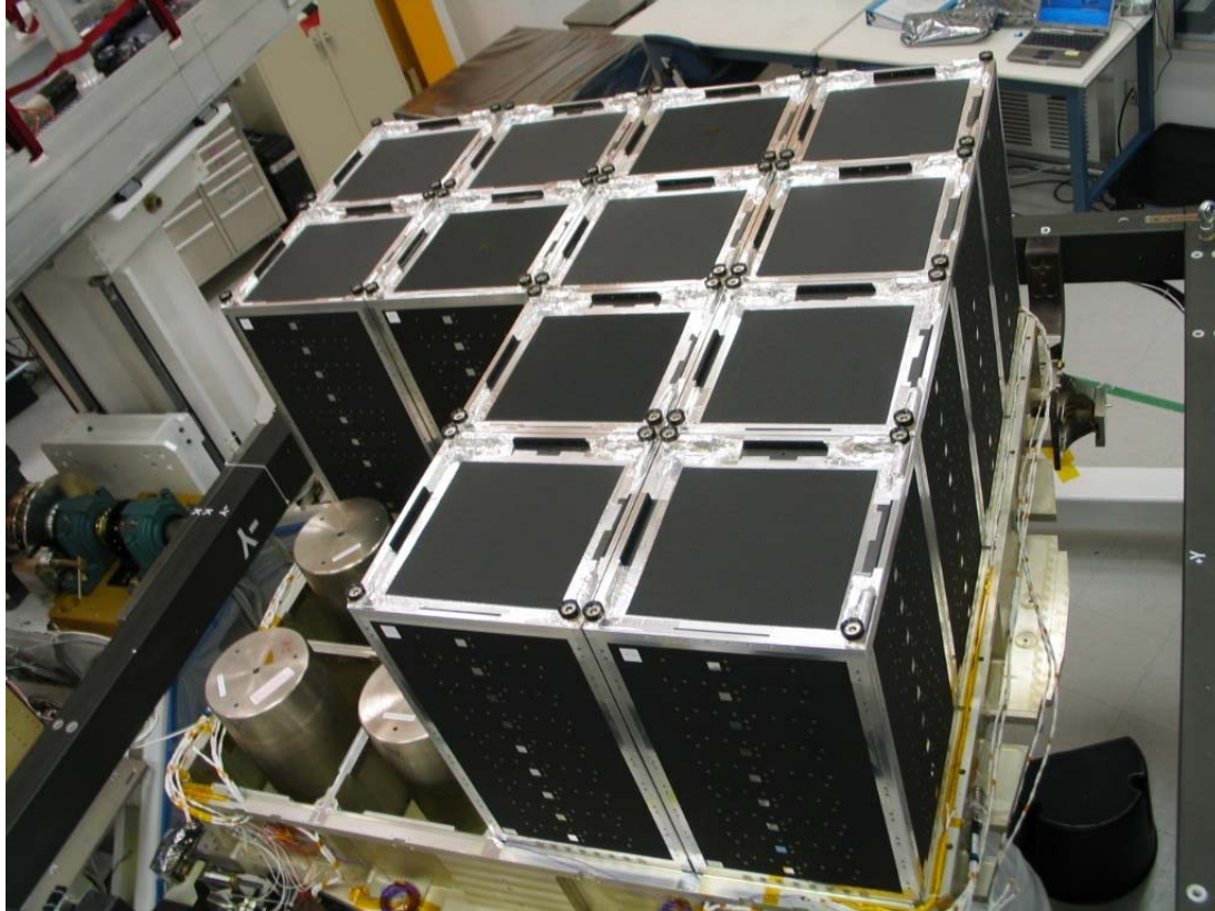
12 towers installed in the grid
