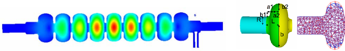
Figure 11 (Left) Field pattern of a trapped mode in the ILC LL cavity with little fields in the end cells, (Right) design variables of the end cell and the optimized (red) vs. original (purple) geometry.
