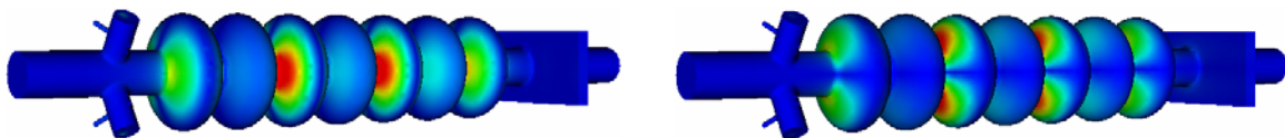
Figure 5: (Left) Low Q_{\text{ext}} polarization of a dipole mode in JLab's 7-cell cavity, (right) high Q_{\text{ext}} polarization of same mode causing the BBU instability.
