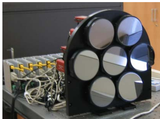
First multi-crystal component of new analyzer crystals for the various proposed applications related to biological and transition metal systems.
