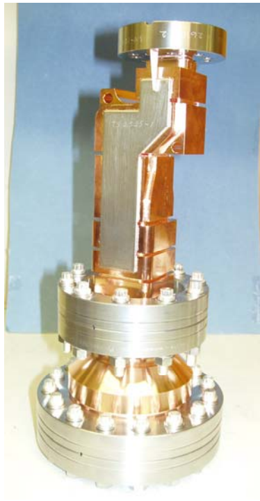
Figure 28: Copper cavity for superconducting materials testing. The bottom flange holds the test sample. Attached to the cavity is the TE_{01} mode launcher described above, through which it is coupled.
