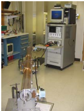
Figure 19: Microwave measurement of an S-band TW structure for LCLS structure.
