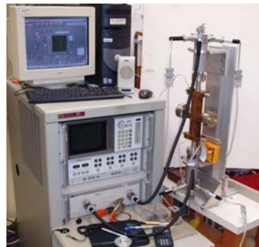
Figure 20: Wire measurement set-up with a SW structure.
