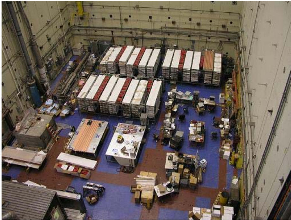
Fig. 16: LSTs under continuous test. These LSTs will be installed in the remaining four barrel sextants during the Summer 2006 shutdown.
