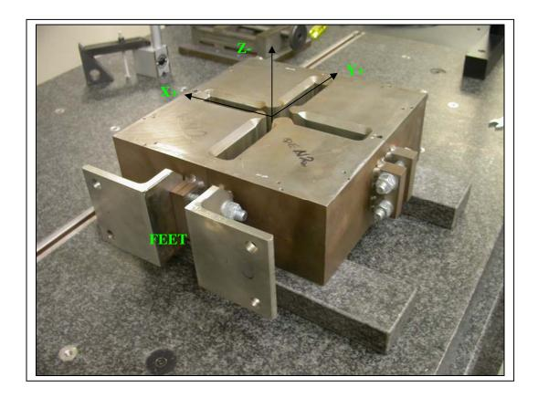
Z zero is set by the mid-plane of the top surface and bottom surface or, the granite parallels.
