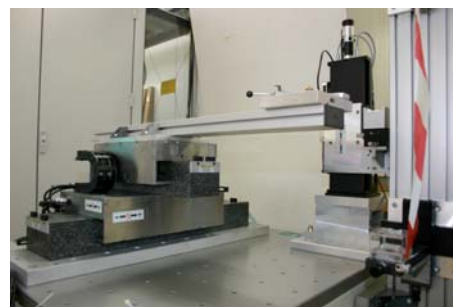
Figure 4: Stretched wire system for the measurement of magnet block inhomogeneities.
