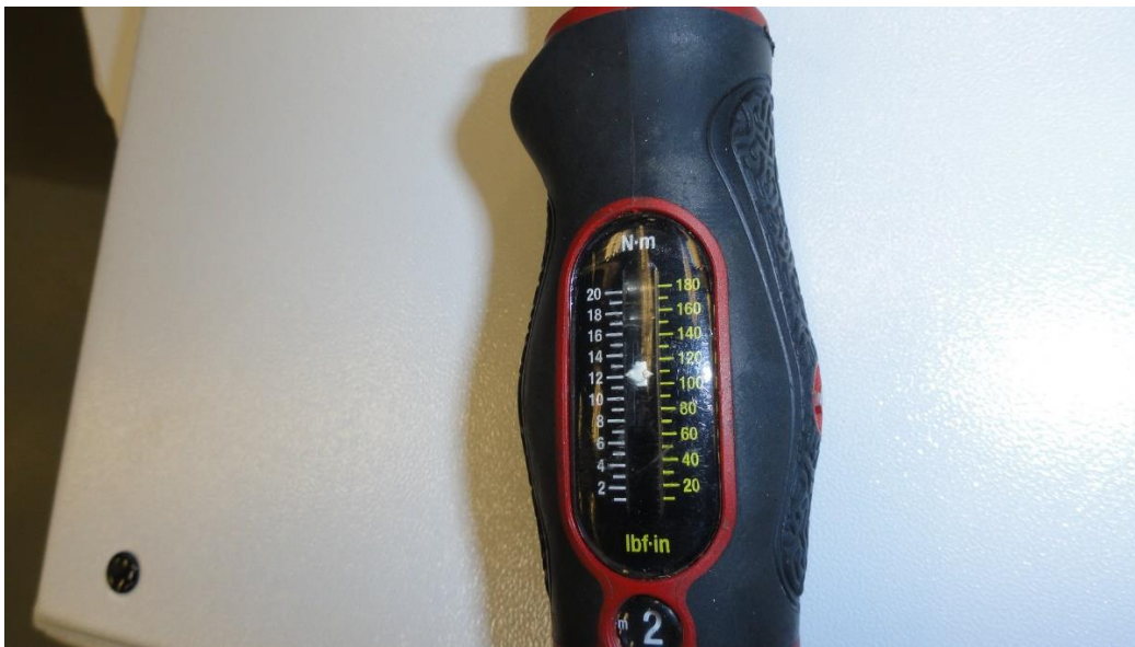
Torque setting for M8 screws (12.2 N-m)
