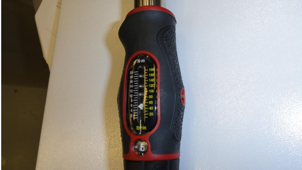
Torque setting for M6 screws (5.6 N-m)
