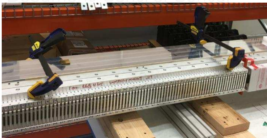
Figure 27: Non-ferrous, soft, rubberized clamps used to keep module on strongback (Exit module pictured).
