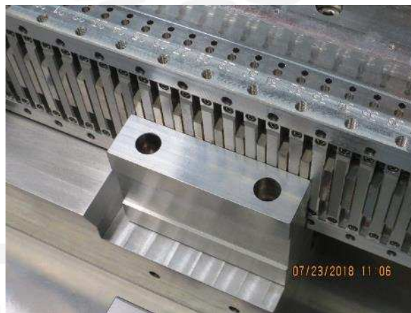
Figure 53: Strongback against gap centering fixture.
