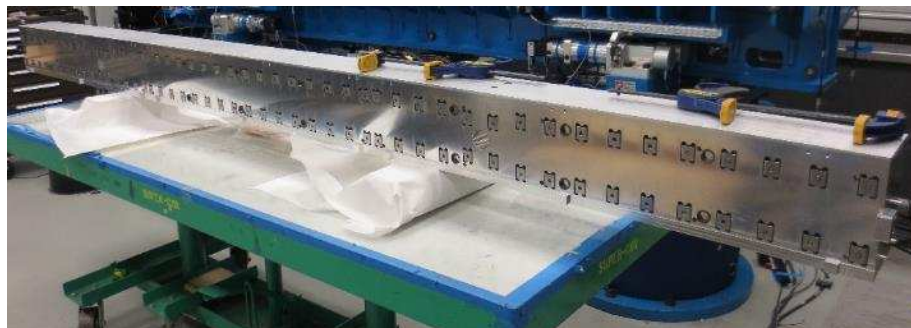
Figure 20: Strongback in upright position, resting on blocks
