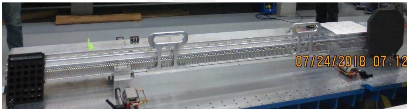
Figure 55: Foam to protect during crane operation of second strongback.
