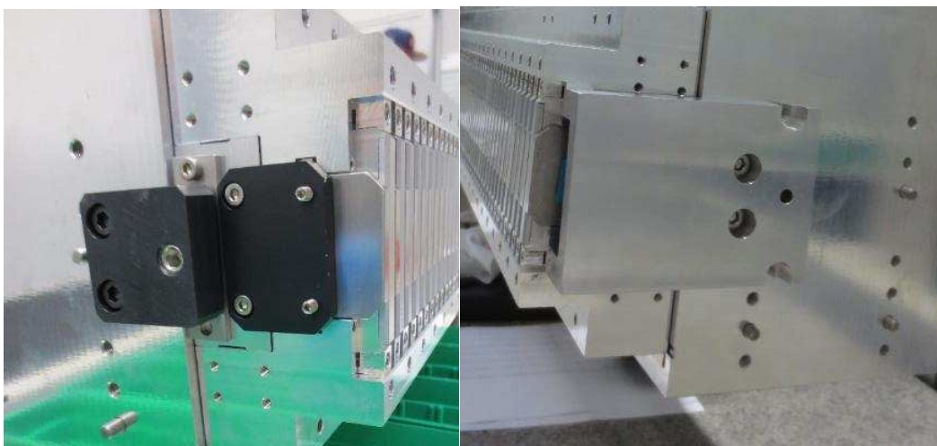
Figure 42: Install end fixtures to keep the Z-position every time modules are loosened.
