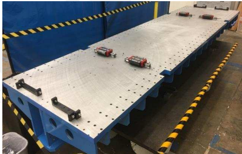
Figure 19: Four hard stop bases installed on pre-production girder.
