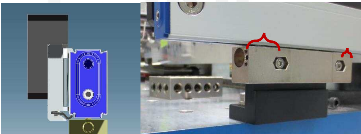
Figure 62: Encoder mounted on backing plate (left) Connector faces out, connector is side with screw further from edge (right).
