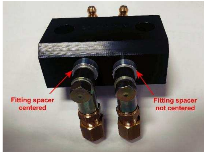
Figure 57: Ensure grease fitting spacer is centered.
