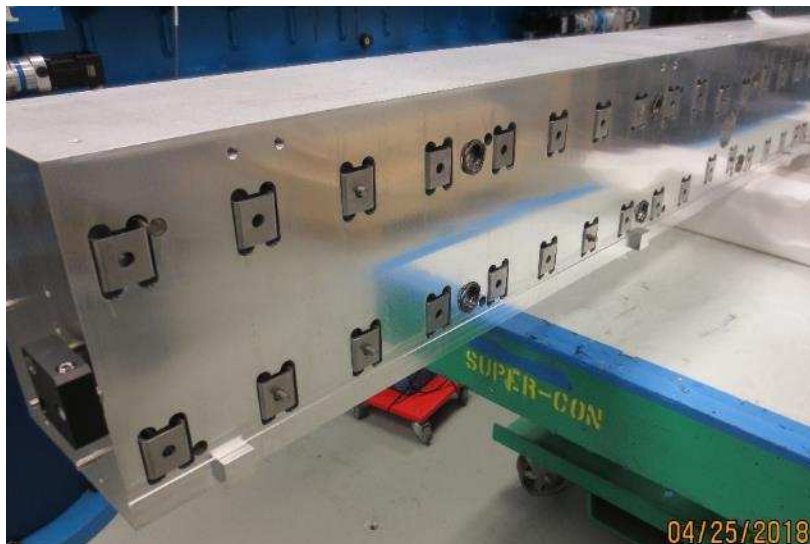
Figure 22: Box flexures, nested springs and bolts inserted.
