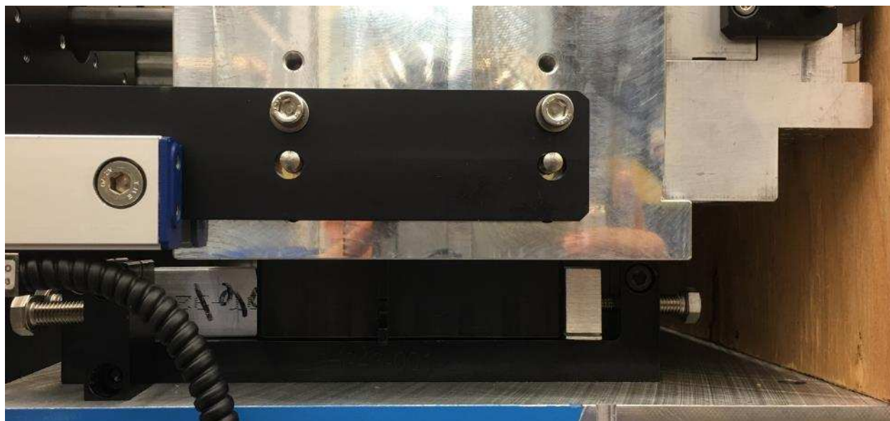
Figure 54: Blocks in the hardstop keeping strongback towards center.
