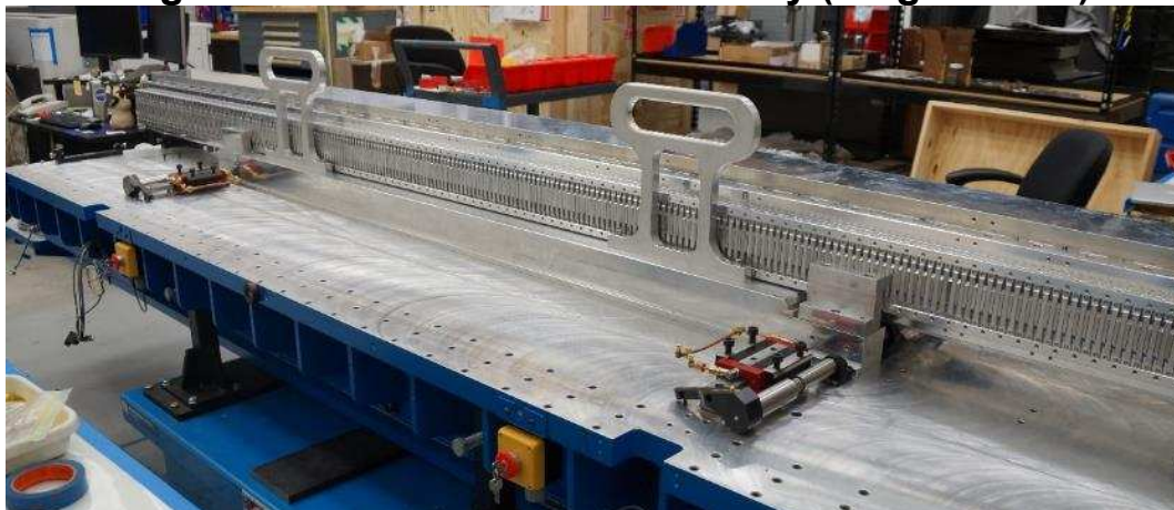
Figure 44: Gap centering fixture and one strongback on girder.
