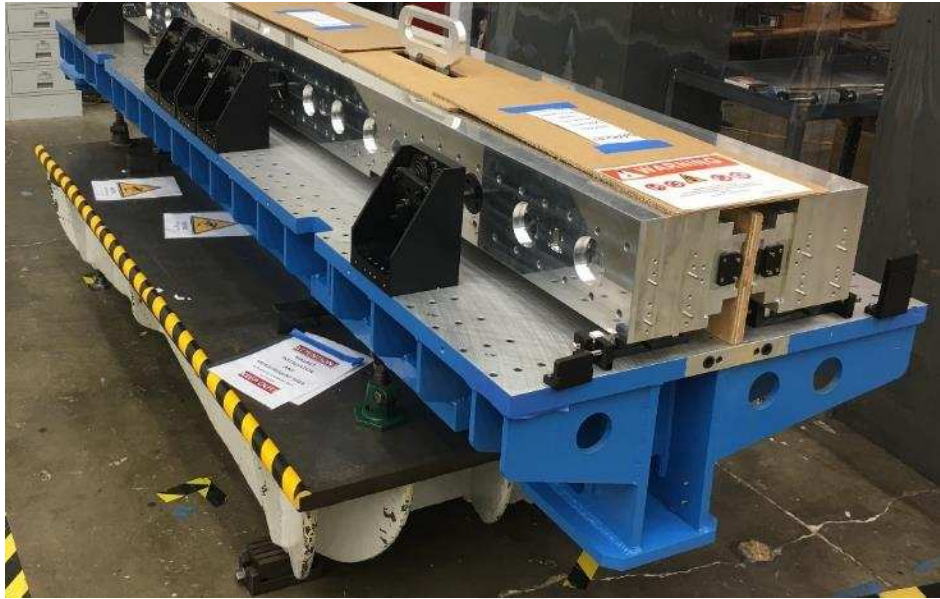
Figure 7: Pre-production undulator supported on the beam running the length of the bottom with jacks and clamps (not visible).
