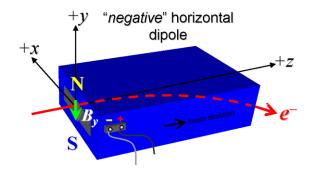
Figure 1. BRLCUS is a "negative" horizontal polarity dipole (bending electrons to the right).
