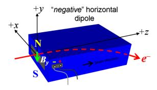
Figure 1. BLRDG0 is a "negative" horizontal polarity dipole (bending electrons to the right).
