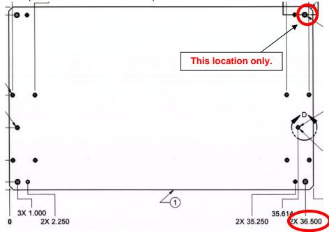
2. With respect to the Waterjet cut, holes near end of length drifted X = -0.009", Y = -0.008".
