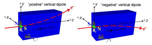
Figure 1. "Positive" polarity (bending electrons up). "Negative" polarity (bending electrons down).
