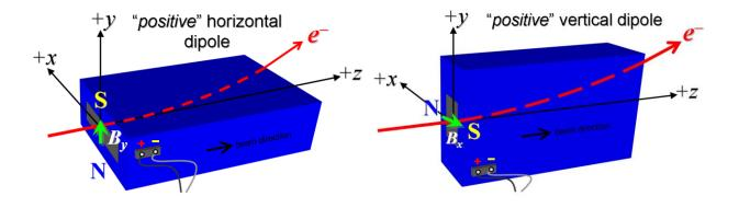
Figure 1. BRCUS1 is "positive" polarity (bending electrons left).
