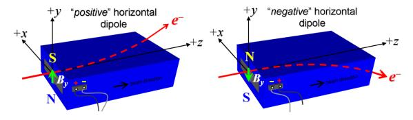
Figure 1. "Positive" polarity (bending electrons up). "Negative" polarity (bending electrons down).
