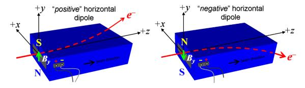
Figure 1. "Positive" polarity (bending electrons left) . "Negative" polarity (bending electrons right).
