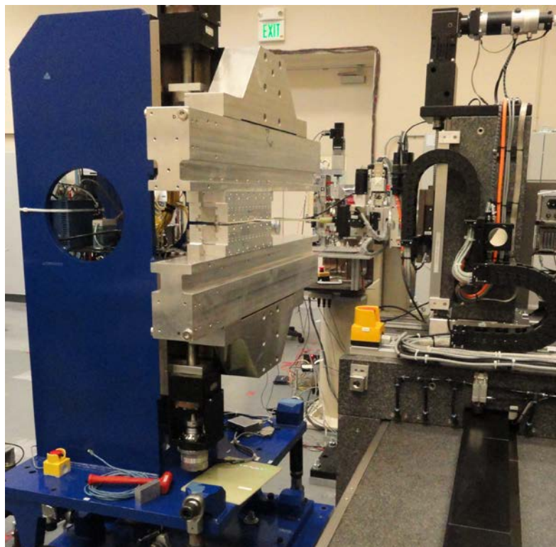
Figure 1. Hall probe measurement setup for the short prototype. The short magnet modules are mounted on the 1 m short frame from the LCLS-II project.
