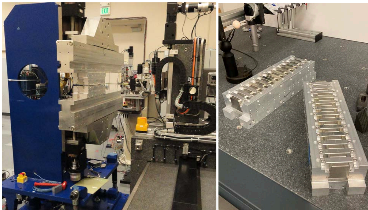
Figure 1. Hall probe measurement setup for the short prototype (left) and short magnet modules after final assembly (right). The short magnet modules are mounted on the 1 m short frame from the LCLS-II project.
