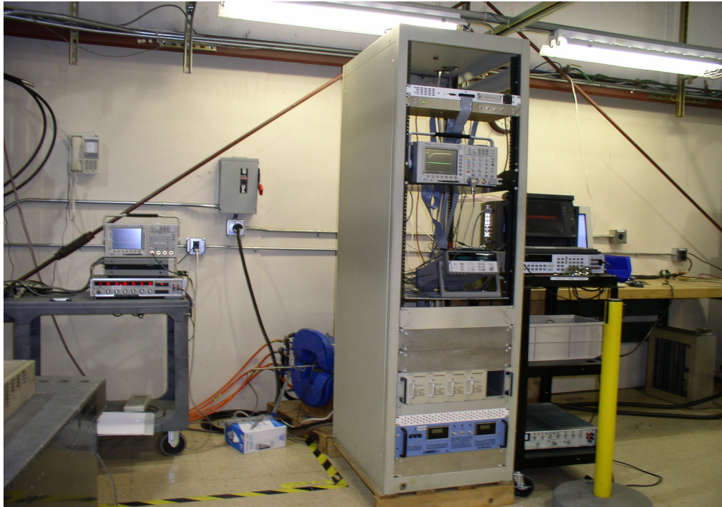
Fig. 1 Measurement Setup: Cart with Hall Probe Power Supply, Amplifier at left; O.C.E.M. Power Supply in rack at right. In this position, the Hall Probe signal is not depressed when switching occurs. If the cart is moved to the front and closer to the rack, the Hall probe signal after switching is depressed.
