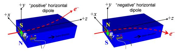
Figure 1: "edge" dipoles SA-257-060-40 are "positive" (left), while "center" dipoles SA-257-060-44 are "negative" (right).
