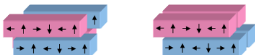
Figure 1. Shift modi of a fixed gap APPLE II: phase shift \phi with pairwise shifts of diagonal magnet arrays (left) and energy shift \rho with shift top versus bottom (right).
