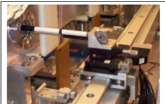
Fig. 25 Arcing rod attached to cross slide
