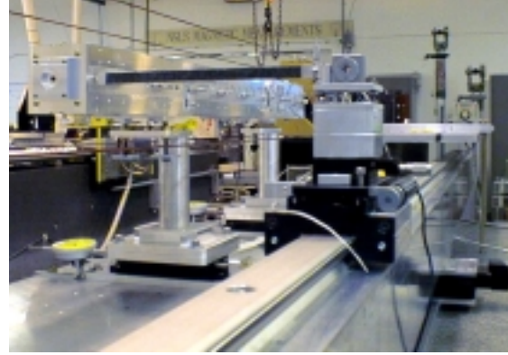
Fig. 34 Bench with undulator magnet and interferometer set-up
