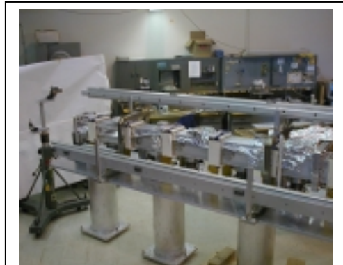
Fig. 21 VISA test installation with jig
