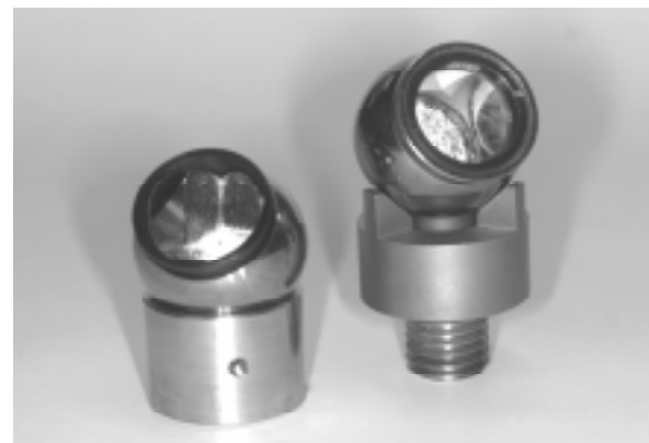
Fig. f711_d Sphere mounted glass and air reflectors
