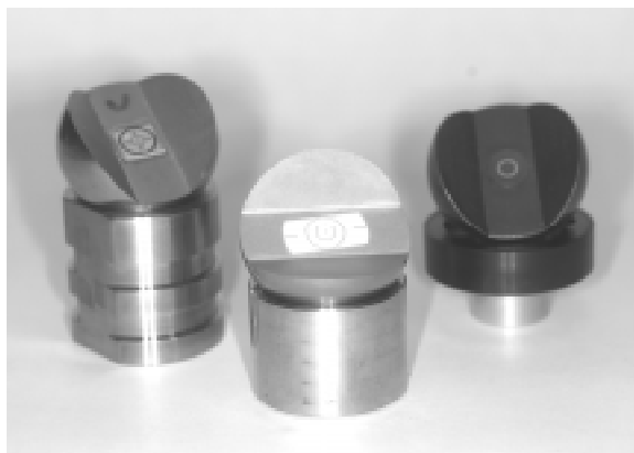
Fig. f711_c Sphere mounted theodolite target
