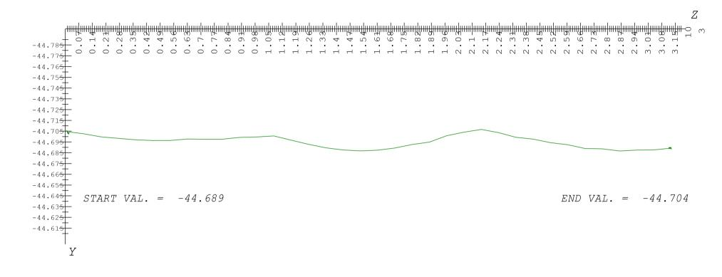
The Start Val. and End Val. are the average of the first and last 15mm of the surface
