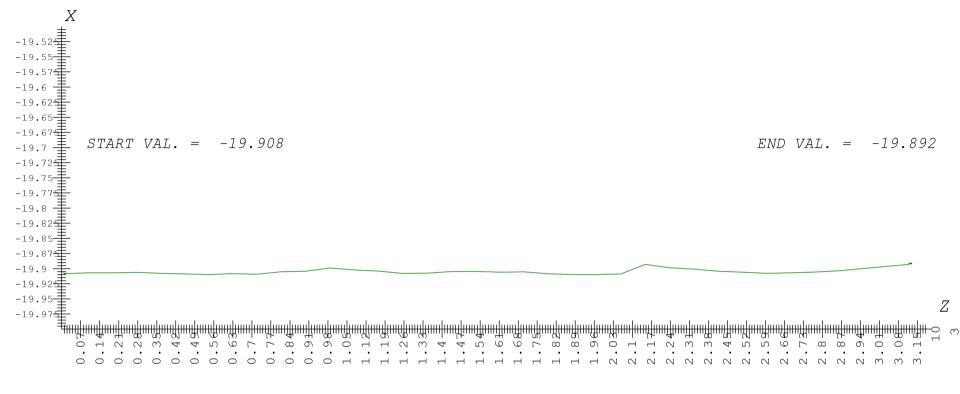
The Start Val. and End Val. are the average of the first and last 15mm of the surface
