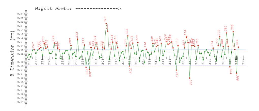
MEAN= 0.043 MIN= -0.078 MAX= 0.213 Labeled Magnets are outside of +/-.05mm from centerline
