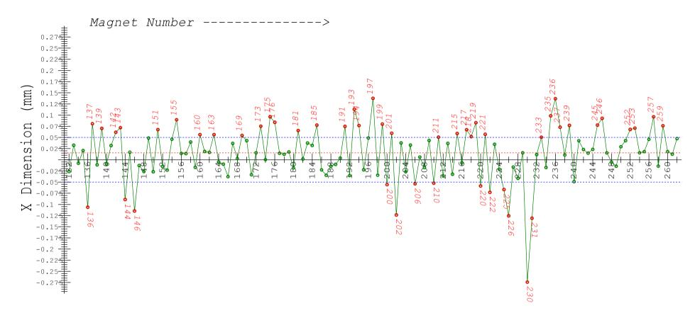
MEAN= 0.015 MIN= -0.124 MAX= 0.138 Labeled Magnets are outside of +/-.05mm from centerline
