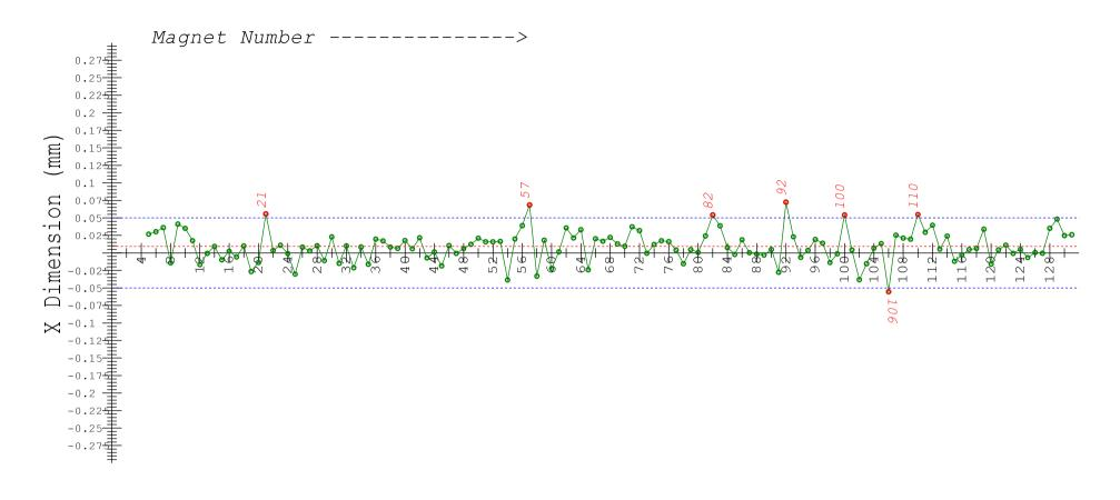
MEAN= 0.009 MIN= -0.038 MAX= 0.072 Labeled Magnets are outside of +/-.05mm from centerline
