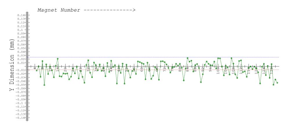
MEAN= -0.009 MIN= -0.051 MAX= 0.023 Labeled Magnets are above .025mm height limit
