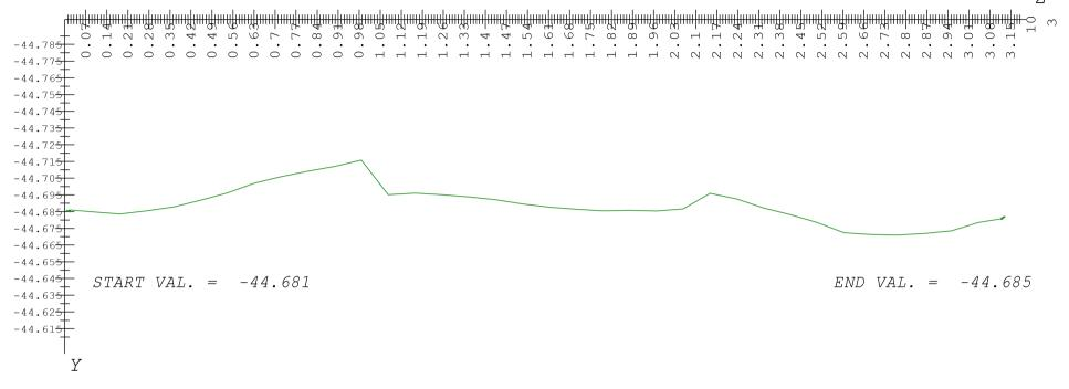
The Start Val. and End Val. are the average of the first and last 15mm of the surface
