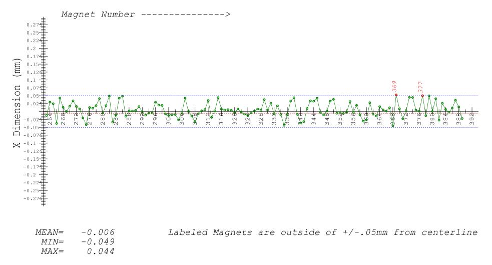
X Axis values have been reversed from measurement csy to be consistant with Keyence sensor
