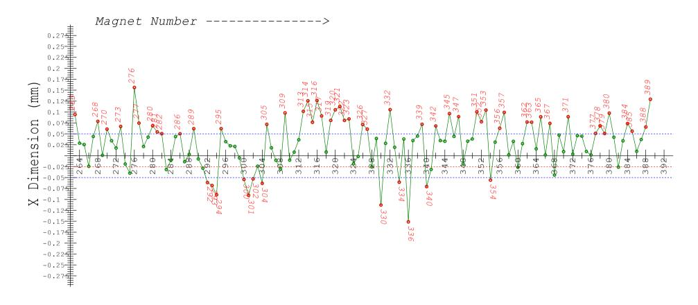
MEAN= -0.025 MIN= -0.156 MAX= 0.151 Labeled Magnets are outside of +/-.05mm from centerline
