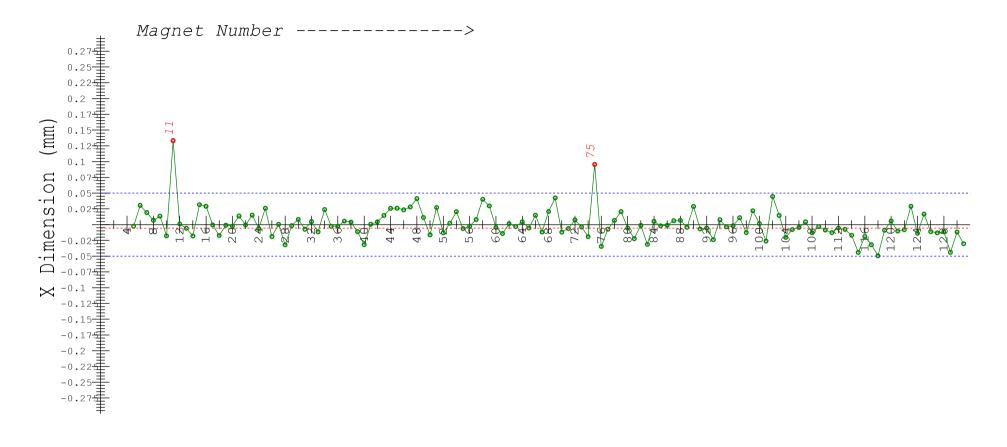
MEAN= -0.006 MIN= -0.133 MAX= 0.035 Labeled Magnets are outside of +/-.05mm from centerline
