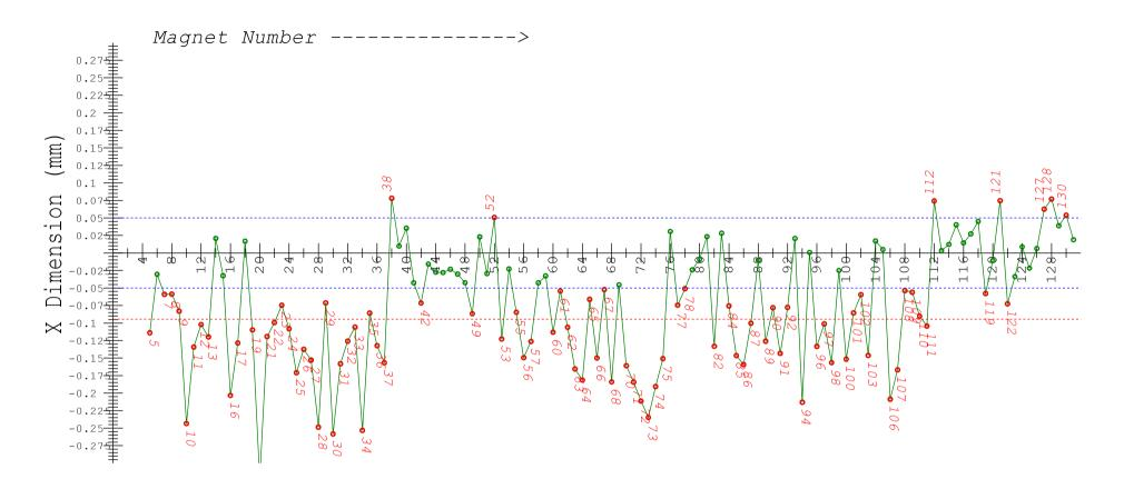
MEAN= -0.095 MIN= -0.325 MAX= 0.078 Labeled Magnets are outside of +/-.05mm from centerline
