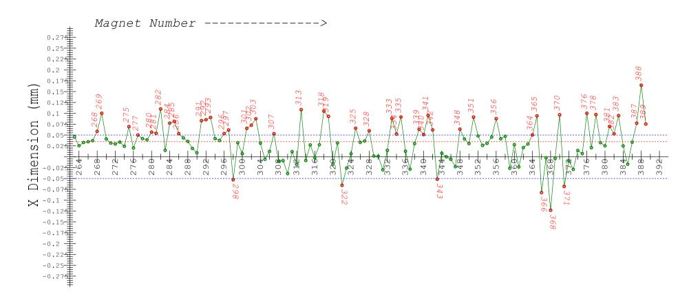
MEAN= 0.035 MIN= -0.066 MAX= 0.110 Labeled Magnets are outside of +/-.05mm from centerline
