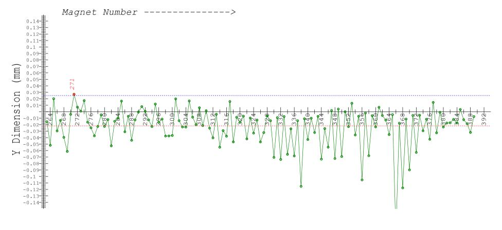
MEAN= -0.022 MIN= -0.115 MAX= 0.027 Labeled Magnets are above .025mm height limit
