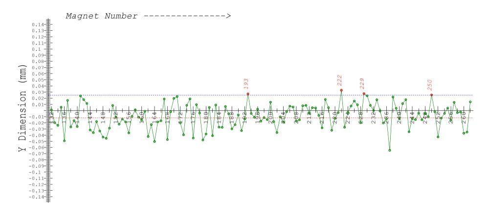
MEAN= -0.012 MIN= -0.050 MAX= 0.033 Labeled Magnets are above .025mm height limit
