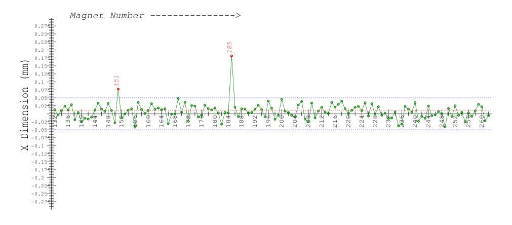
MEAN= 0.011 MIN= -0.042 MAX= 0.181 Labeled Magnets are outside of +/-.05mm from centerline
