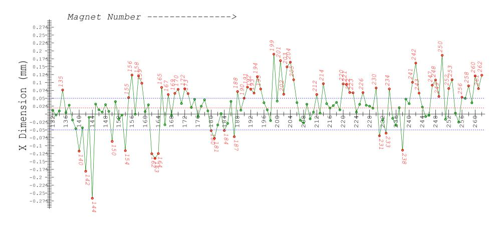
MEAN= 0.020 MIN= -0.266 MAX= 0.190 Labeled Magnets are outside of +/-.05mm from centerline
