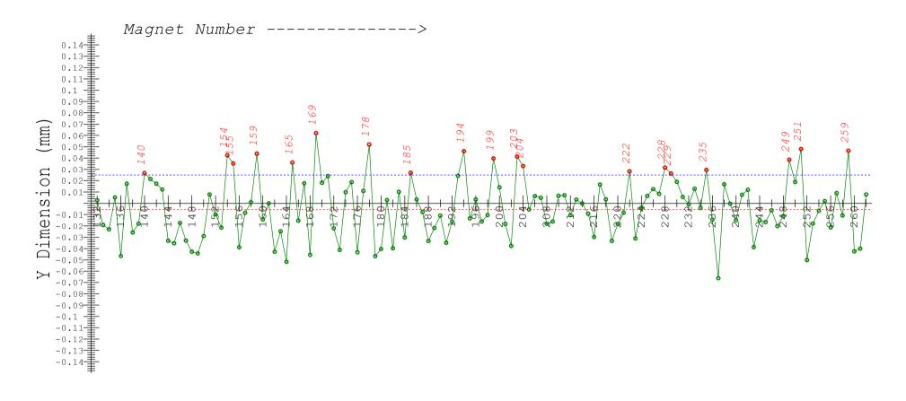
MEAN= -0.006 MIN= -0.052 MAX= 0.062 Labeled Magnets are above .025mm height limit
