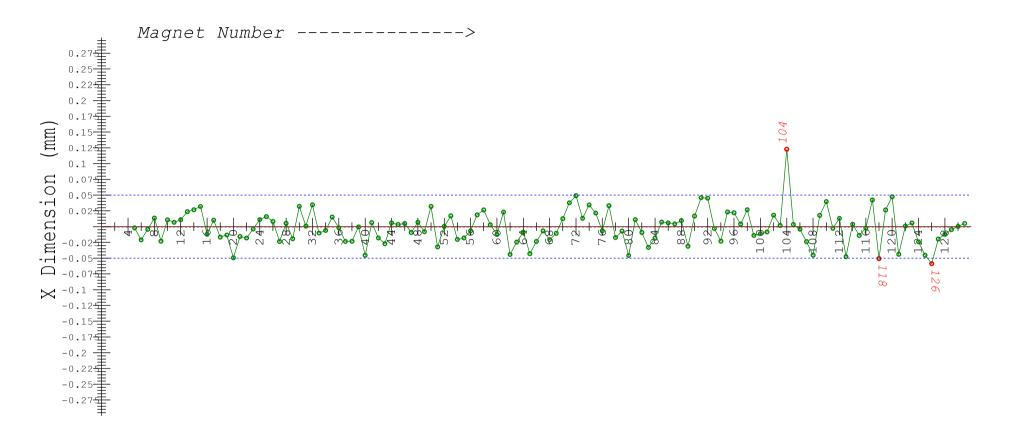
MEAN= -0.001 MIN= -0.049 MAX= 0.049 Labeled Magnets are outside of +/-.05mm from centerline
