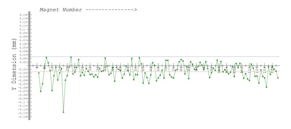
MEAN= -0.016 MIN= -0.128 MAX= 0.023 Labeled Magnets are above .025mm height limit
