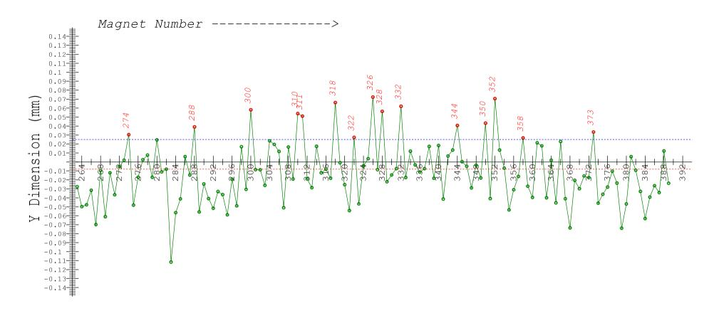
MEAN= -0.008 MIN= -0.112 MAX= 0.072 Labeled Magnets are above .025mm height limit
