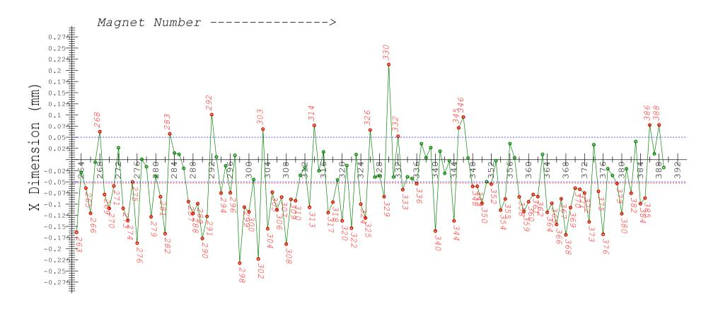
MEAN= -0.053 MIN= -0.232 MAX= 0.213 Labeled Magnets are outside of +/-.05mm from centerline
