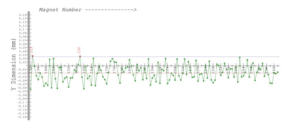
MEAN= -0.020 MIN= -0.063 MAX= 0.027 Labeled Magnets are above .025mm height limit
