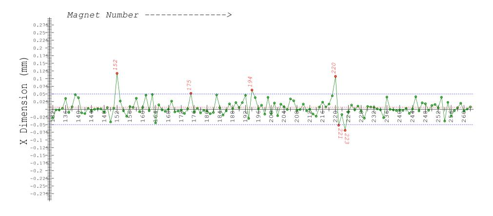
MEAN= 0.007 MIN= 0.117 MAX= -0.069 Labeled Magnets are outside of +/-.05mm from centerline
