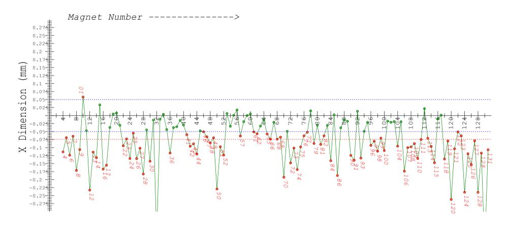
MEAN= -0.074 MIN= -0.382 MAX= 0.058 Labeled Magnets are outside of +/-.05mm from centerline
