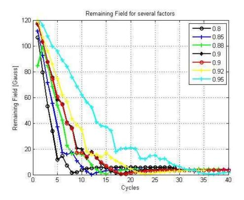
Figure 1: Remaining integrated field after cycles of degaussing.
