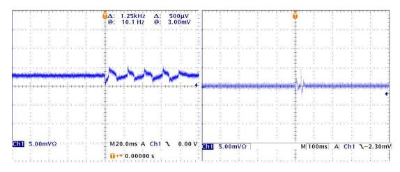
Figure 5: Current Spikes when turning off bulk power supply of MCOR 12; left: ripple peak-to-peak  $\approx 0.5$ A; right: a spike with peaks at  $\approx -0.3$ , +0.5 A
