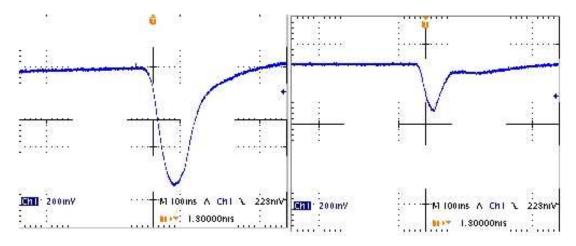
Figure 4: Current Spikes when turning off Power Supply of MCOR Calibration Stand; left: peak current -11A, right: peak current -3.75A
