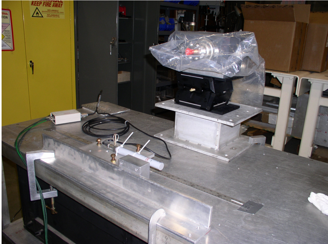
Figure 5. Measurement Setup for the `13 in above 13 in sideways' configuration. Here the pump sits on an additional stand, elevating it 13 inch above the plane of the probe center.
