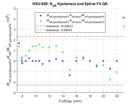
Plotted functions have been calculated from measured values openKeff (opengap) and closeKeff (closegap) using the following Matlab calculations:
